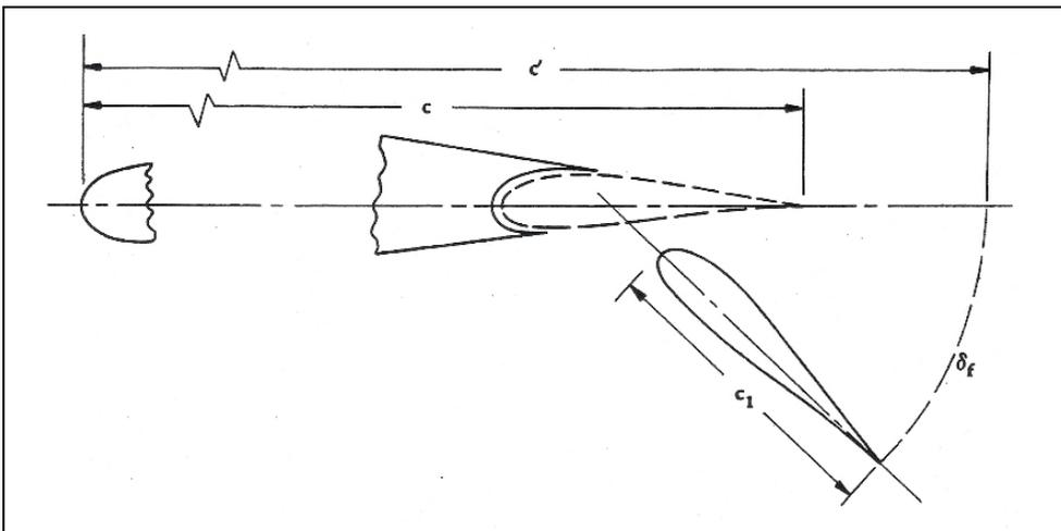
**Fig. 11.11** Definition of Fowler and slotted-flaps geometry (**DATCOM 1978**)
