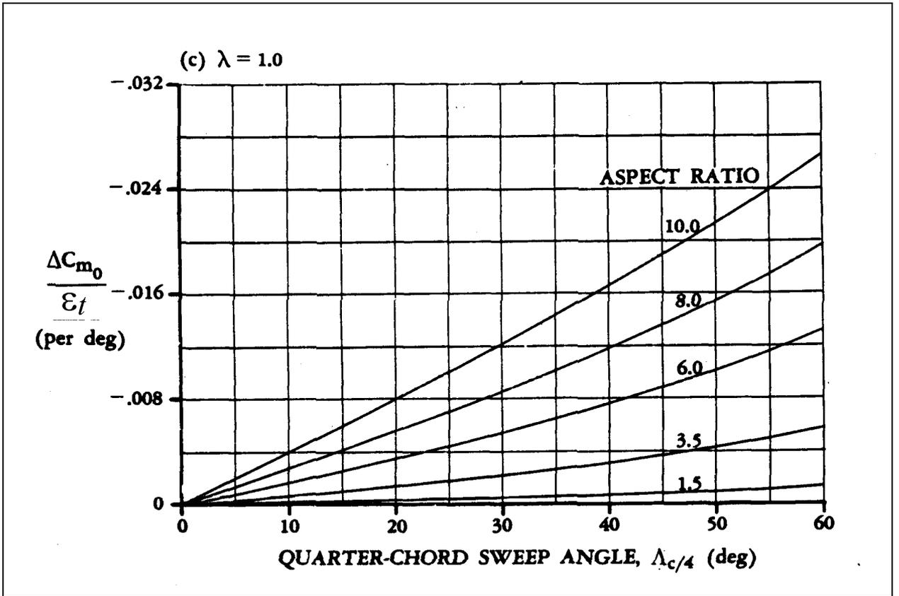
Fig. 11.12b Influence of linear wing twist on pitching moment coefficient with respect to the wing aerodynamic center.  $\Lambda_{c/4}$  stands for quarter-chord sweep angle  $\phi_{25}$  (DATCOM 1978) - Fig. 2 out of 2
