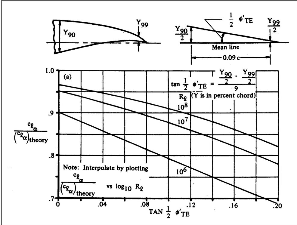
Fig. 11.16  $c_{L,\alpha} / (c_{L,\alpha})_{theory}$  for Fig. 11.15 (DATCOM 1978)
