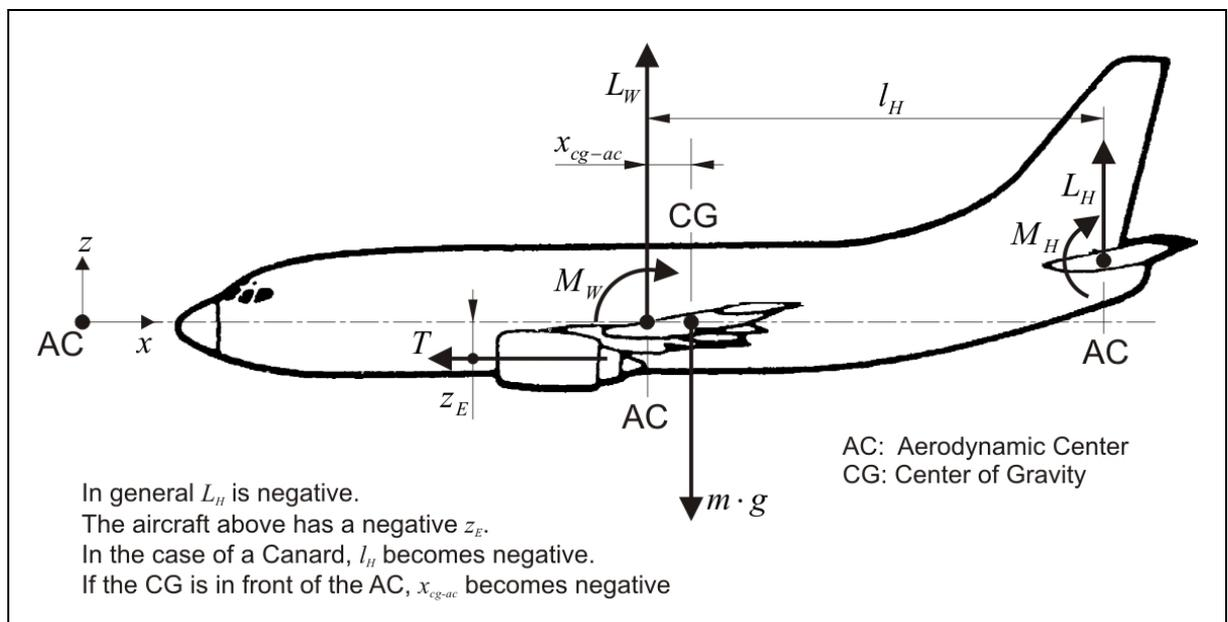
**Fig. 11.1** Forces, moments and lever arms to calculate pitching moment
