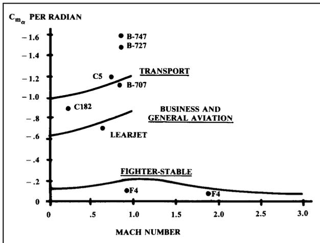
**Fig. 11.6** Typical pitching moment coefficients  $C_{M,\alpha}$  for aircraft design predefinition of static margin (Raymer 1989)
