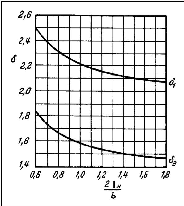
**Fig. 11.10** Diagram for calculation of horizontal tail downwash angle with the help of horizontal tail lever arm  $l_H$  and wing span  $b$  (Dubs 1987)
