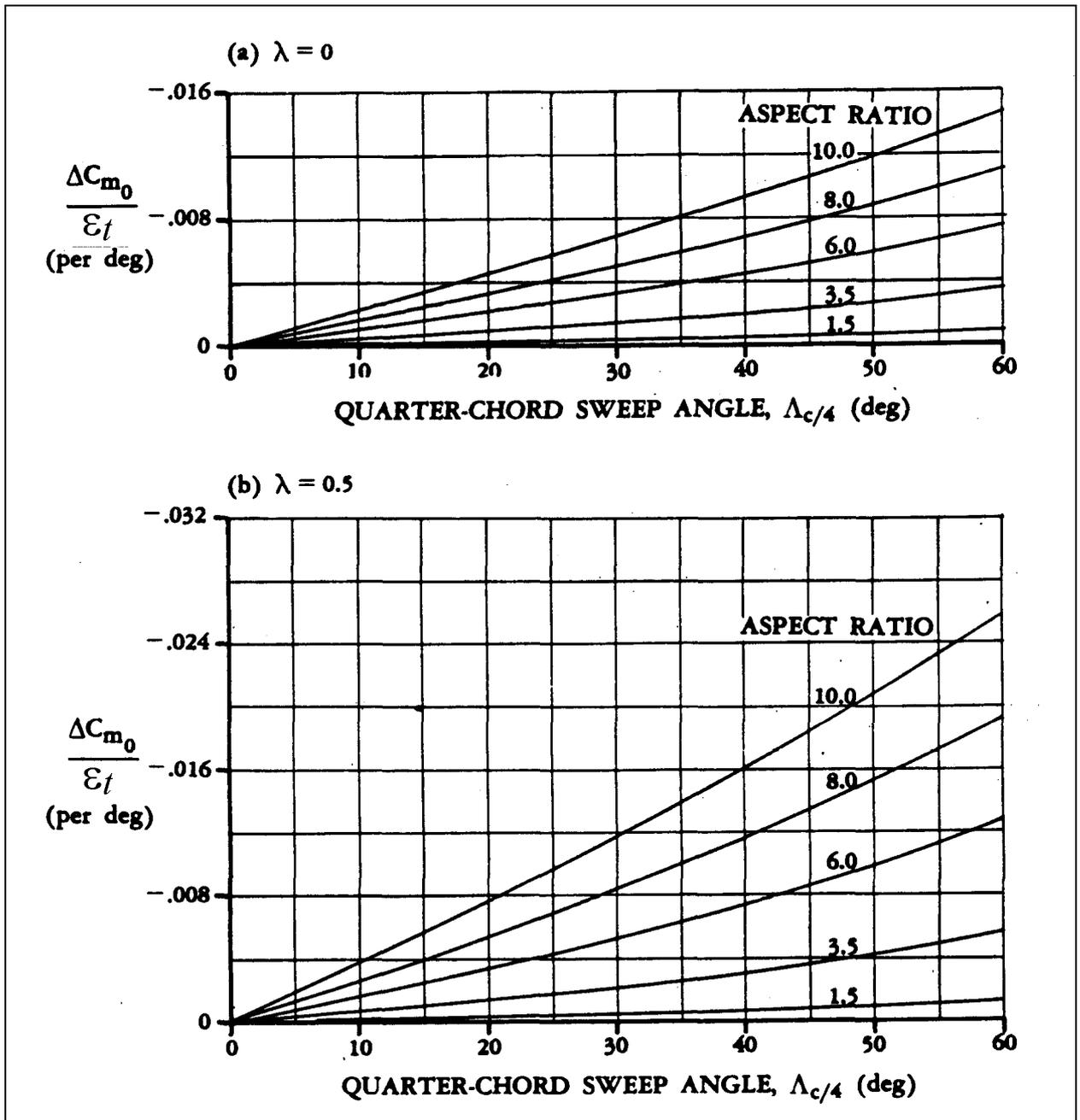
Fig. 11.12a Influence of linear wing twist on pitching moment coefficient with respect to the wing aerodynamic center.  $\Lambda_{c/4}$  stands for quarter-chord sweep angle  $\phi_{25}$ . (DATCOM 1978) - Fig. 1 out of 2
