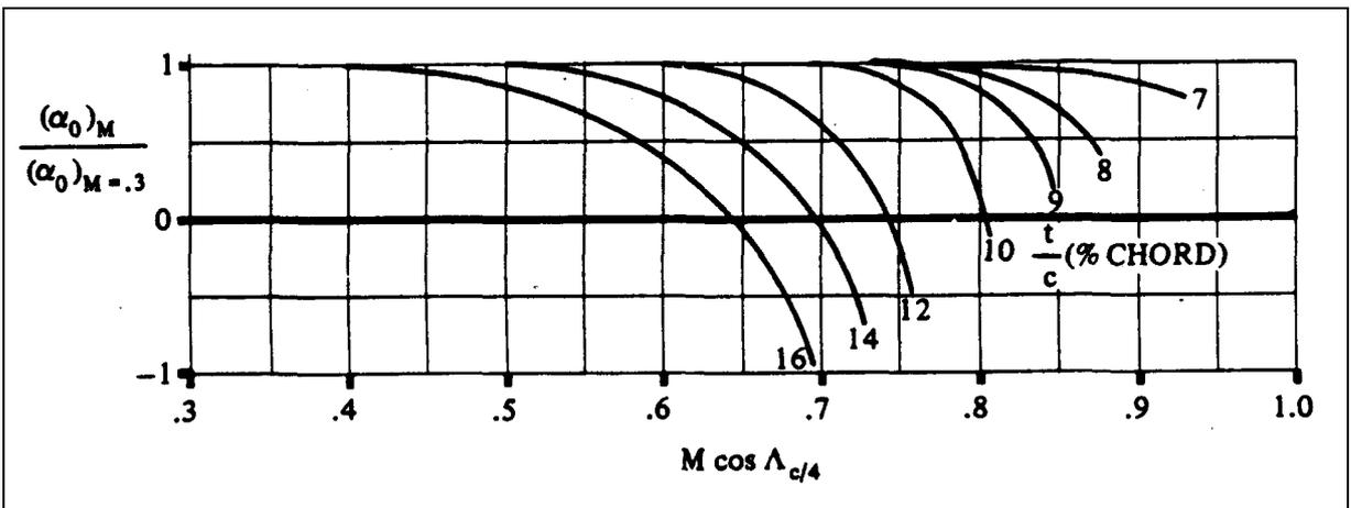
Fig. 11.8 Mach number correction to calculate wing zero lift angle (DATCOM 1978)
