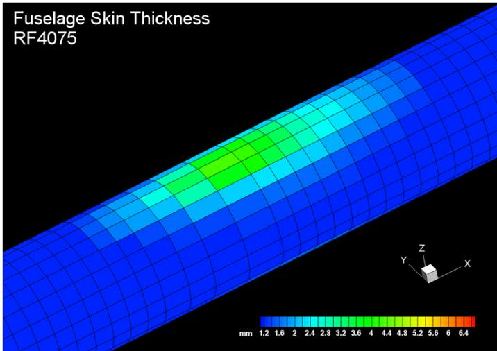
Figure 5.6: Fuselage Skin Thickness of Version RF4075
