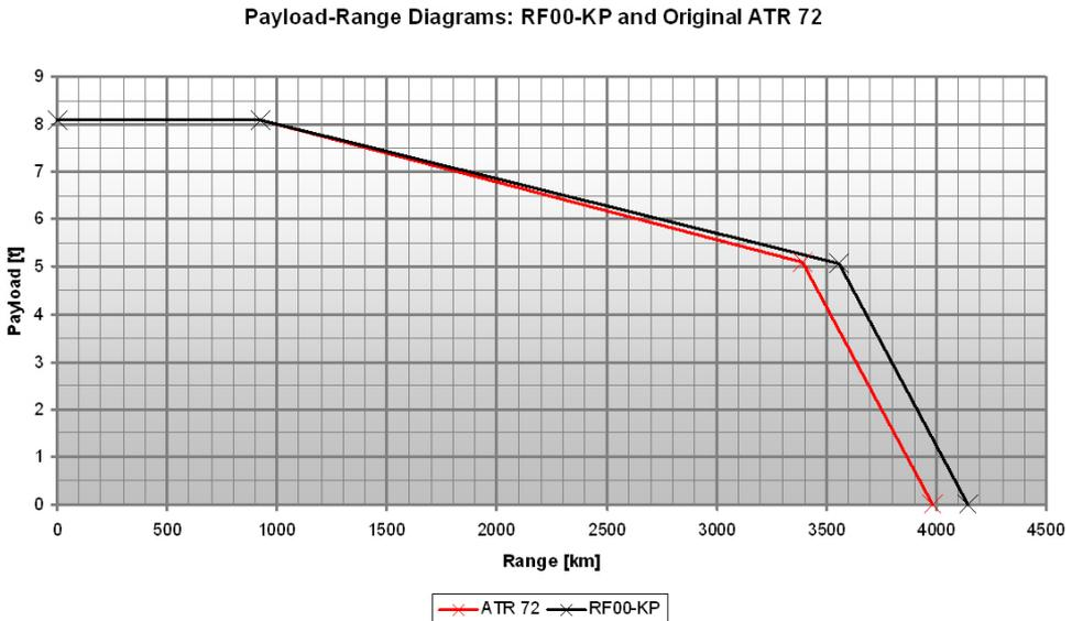
Figure 4.8: Payload-Range Diagrams of RF00-KP and Original ATR 72
