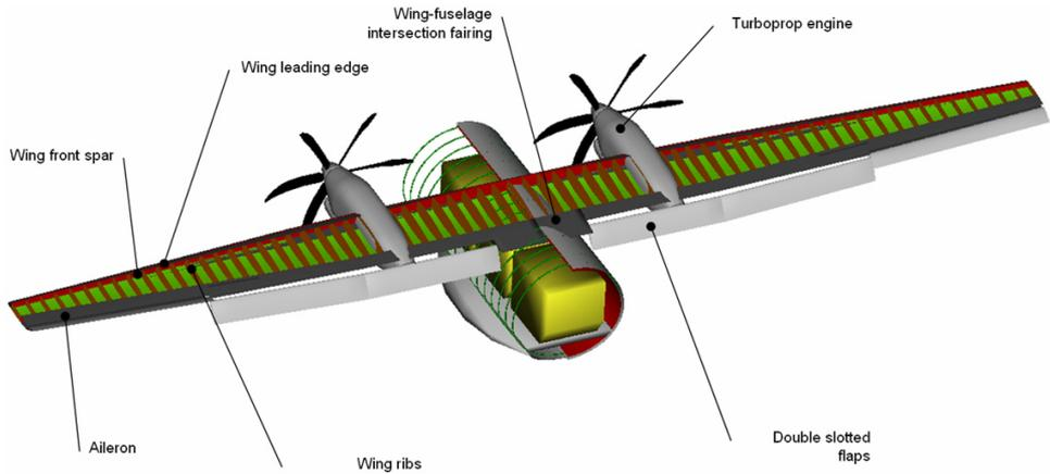
Figure 4.6: Version RF00-KP Wing and Center Fuselage Section
