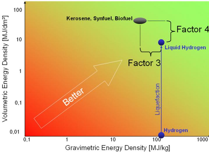
Figure 2.9: Energy Densities of Kerosene and Hydrogen
