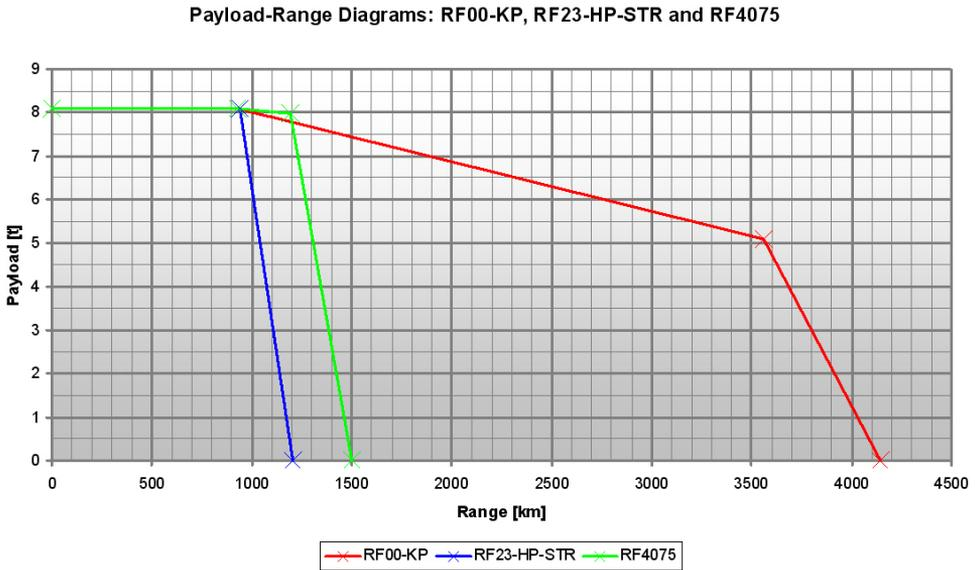
Figure 5.8: Payload-Range Diagrams of RF00-KP, RF23-HP-STR and RF4075
