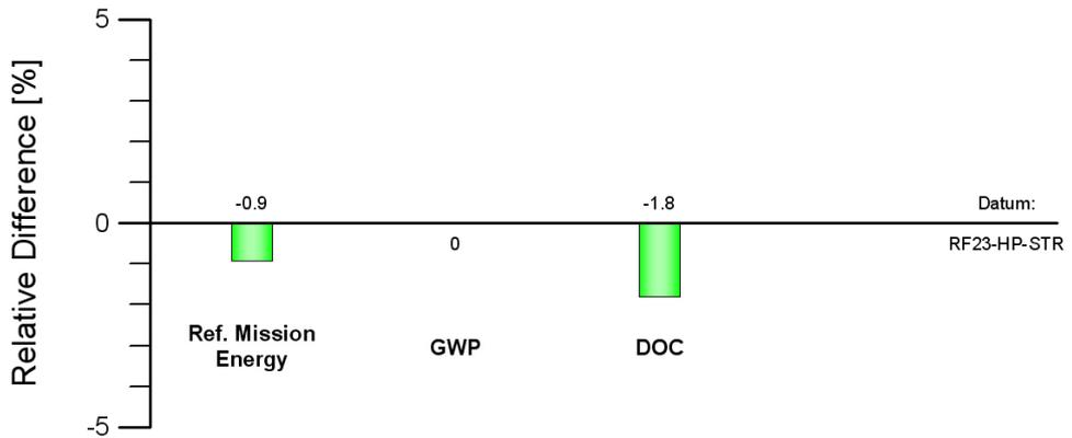
Figure 5.10: Relative Differences in Ref. Mission Energy, GWP and DOC of Version RF4075 to Version RF23-HP-STR
