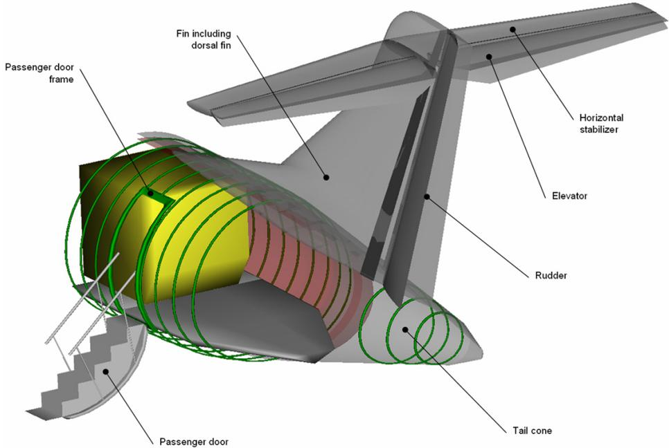
Figure 4.7: Version RF00-KP Tailplane and Rear Fuselage Section
