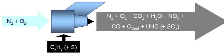
Figure 2.6: Combustion Products of Conventional and Synthetic Kerosene
