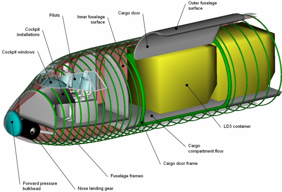
Figure 4.5: Version RF00-KP Forward Fuselage Section
