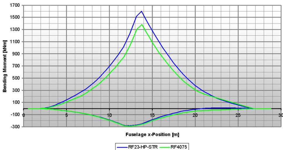
Figure 5.4: Fuselage Beam Model: Bending Moments of Versions RF23-HP-STR and RF4075
