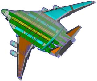
FIG 8. Blended Wing Body with (hybrid) hydrogenpropulsion technology
