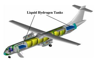
FIG 7. Hydrogen-powered regional cargo aircraft with fuel tanks inside the fuselage
