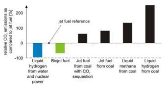
FIG 3. Relative carbon dioxide emissions of different alternative fuels over their whole life-cycle compared to conventional kerosene (based on IATA, 2008)
