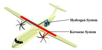
FIG 9. Hybrid-powered demonstrator aircraft
