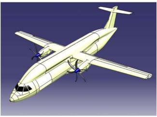
FIG 4. Regional cargo aircraft with fuel stores mounted on top of the fuselage
