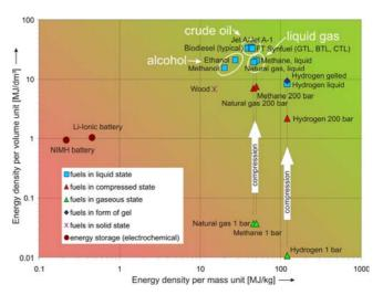
FIG 2. Volumetric and gravimetric energy contents of different fuels and batteries on a double logarithmic scale (based on Sieber, 2009)
