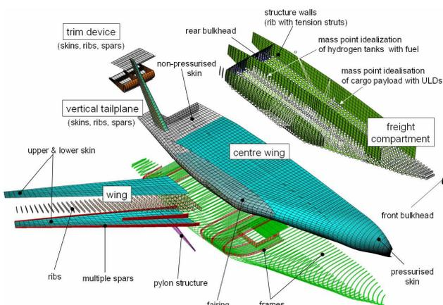
Fig. 3. PrADO SAM-Model for Structural Sizing and Mass Calculation
