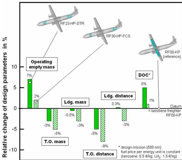
Fig. 6. Relative Comparison of Hydrogen Aircraft Versions and Reference Kerosene Aircraft
