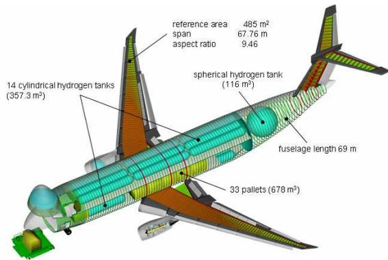
Fig. 7. Optimized Conventional Hydrogen Freighter
