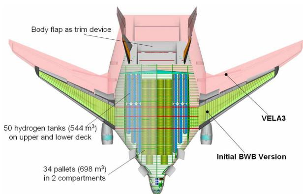
Fig. 8. PrADO Model of Initial BWB Version in Comparison to VELA3 Configuration
