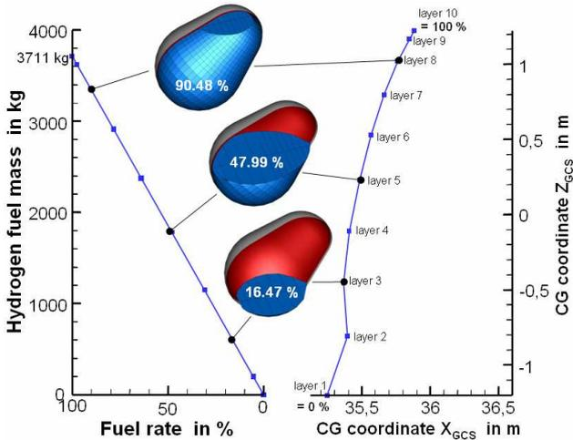
Fig. 1. PrADO Cryogenic Fuel Tank Model
