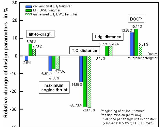
Fig. 11. Relative Comparison of Hydrogen Aircraft Versions and Reference Kerosene Aircraft
