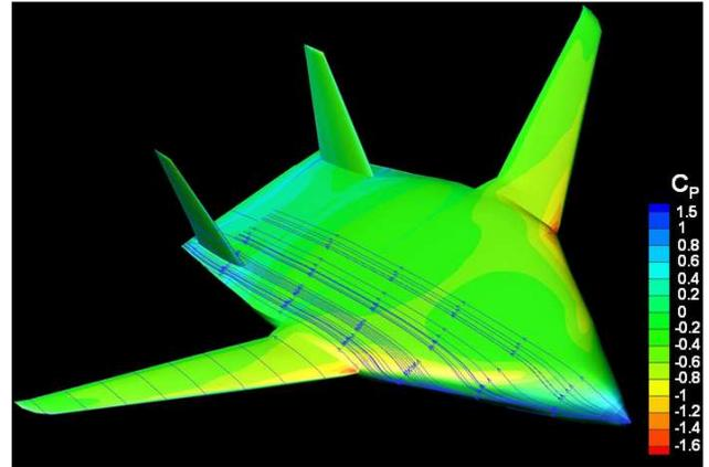
Fig. 4. Pressure Distribution on the Unmanned BWB Aircraft Design for SAM Aerodynamic Load Determination (Panel Code HISSS)
