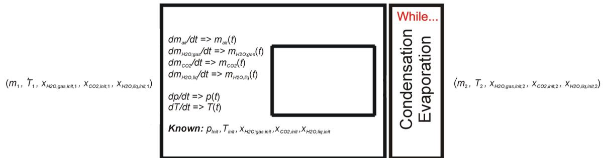
**Figure 12:** Inner structure of a generalized volume with water vapor, CO<sub>2</sub> and free water balance
