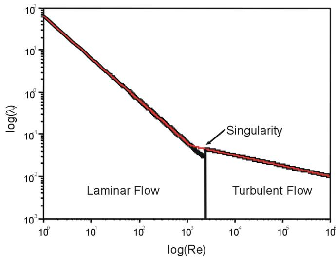
**Figure 15:** The transition between laminar and turbulent flow
