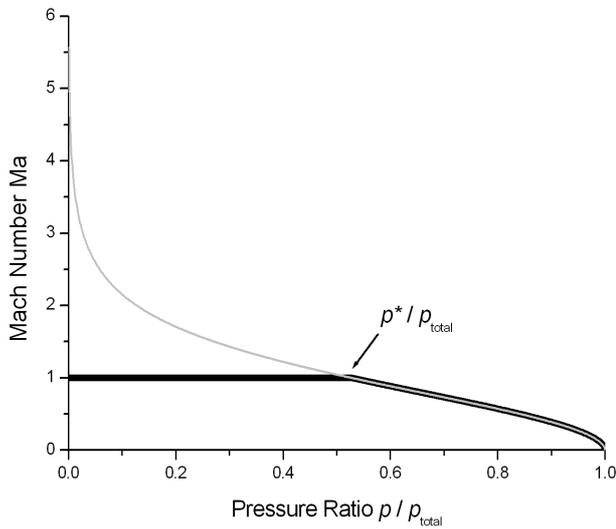
**Figure 19:** Mach number characteristics based on Equation 50
