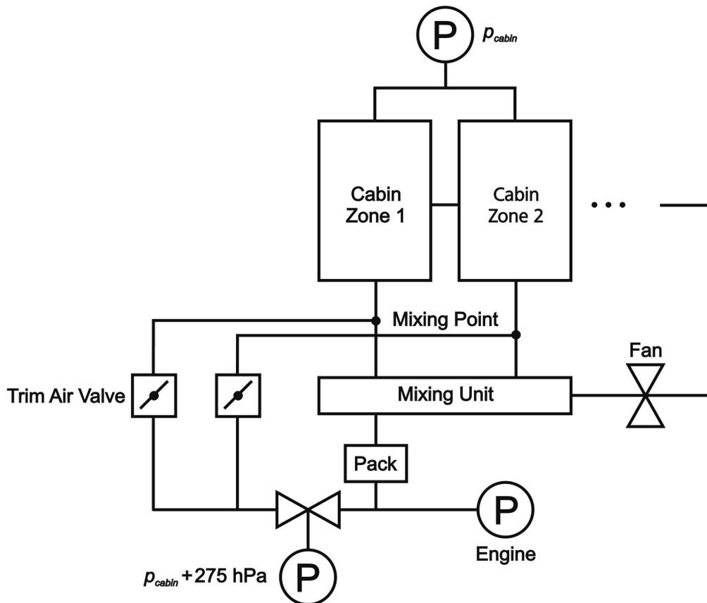
**Figure 2:** Schematic drawing of the environmental control system
