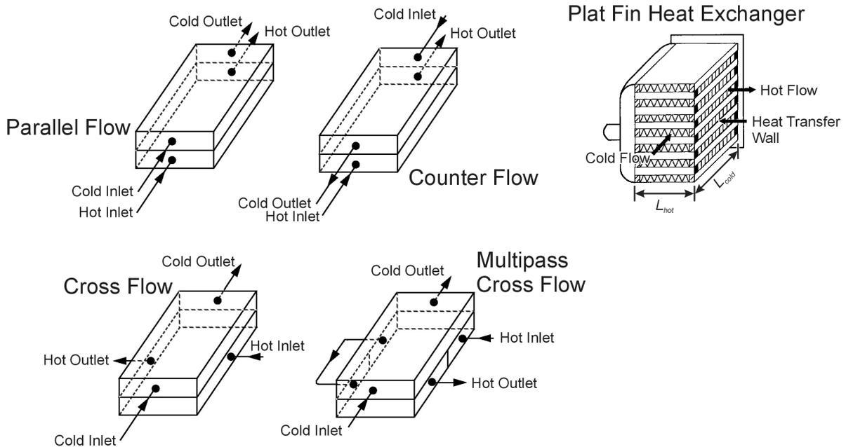
**Figure 24:** Different configuration of heat exchangers (Allied-Signal 1990)
