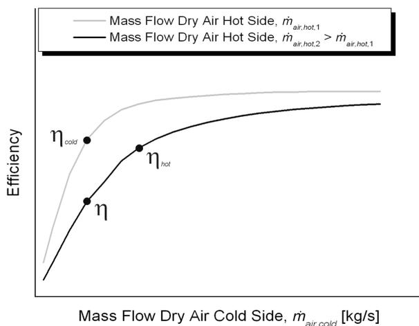
**Figure 25:** Efficiency function of a heat exchanger
