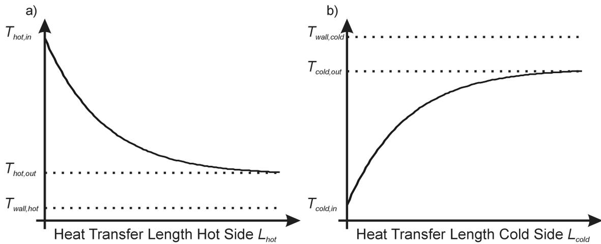
**Figure 27:** a) Hot side: Temperature profile along the contact length
