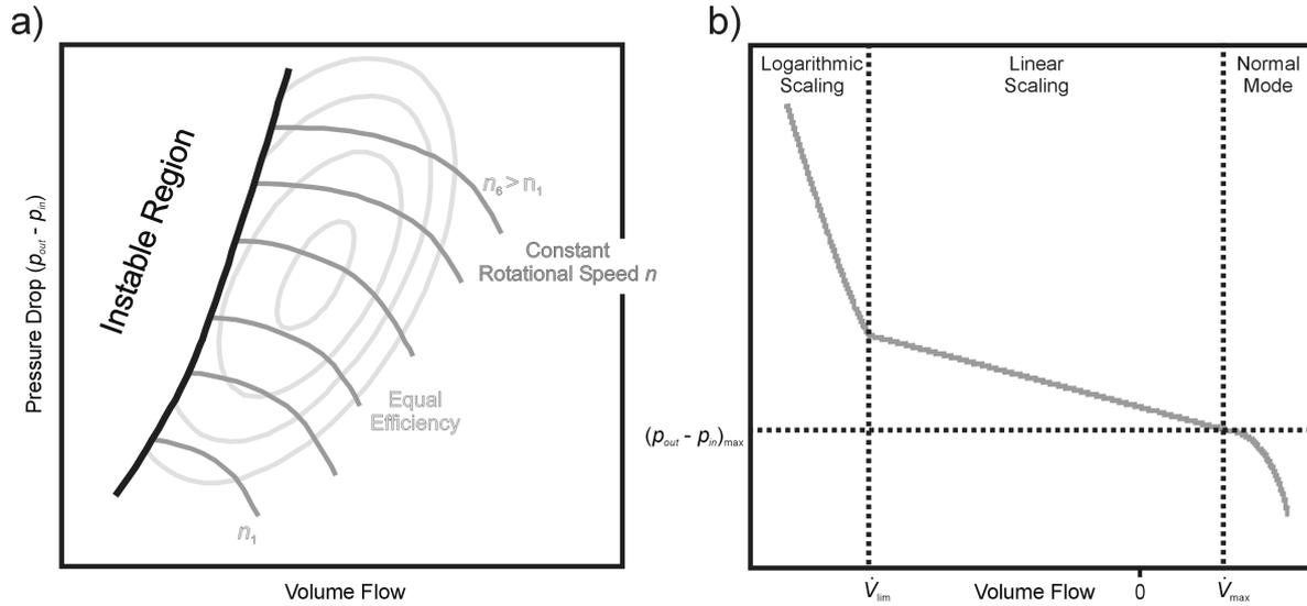
**Figure 29:** a) Characteristic map of a generalized fan
