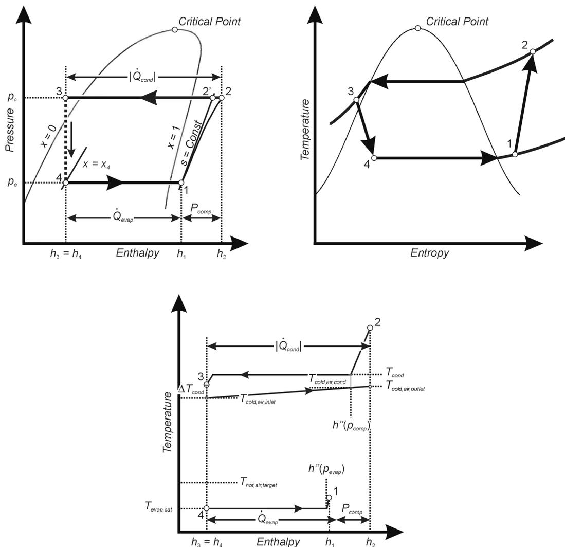
**Figure 36:**  $p-h$ ,  $T-s$  respectively  $T-h$  diagrams of R134a refrigerant
