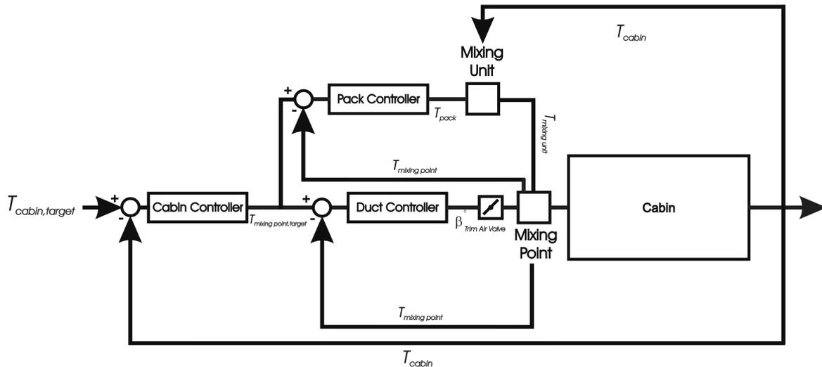
**Figure 3:** The control aspects of a cabin simulation
