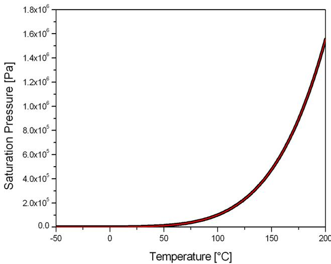
**Figure 11:** The saturation pressure of water vapor in air, as function of the temperature. Black line: measured data, red line: fit function (see text)
