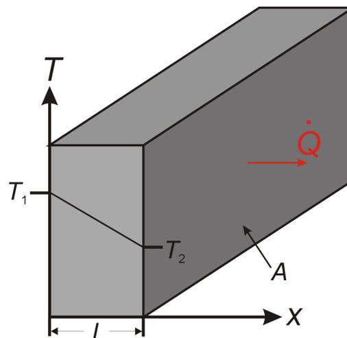
**Figure 20:** Heat conduction
