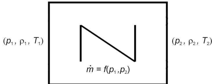
**Figure 14:** Inner structure of a flow resistance
