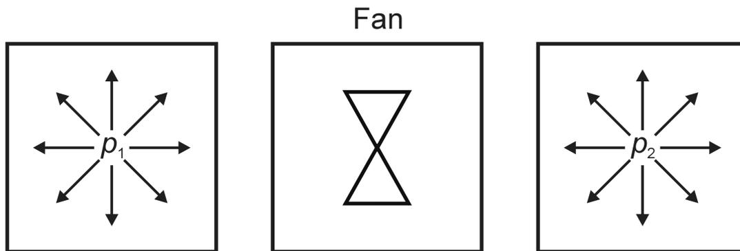
**Figure 28:** Configuration of a fan component as flow resistance
