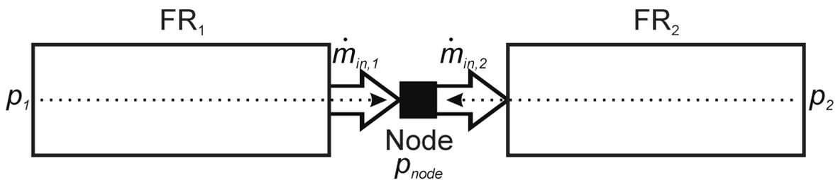
**Figure 16:** Node between to flow resistance (FR)
