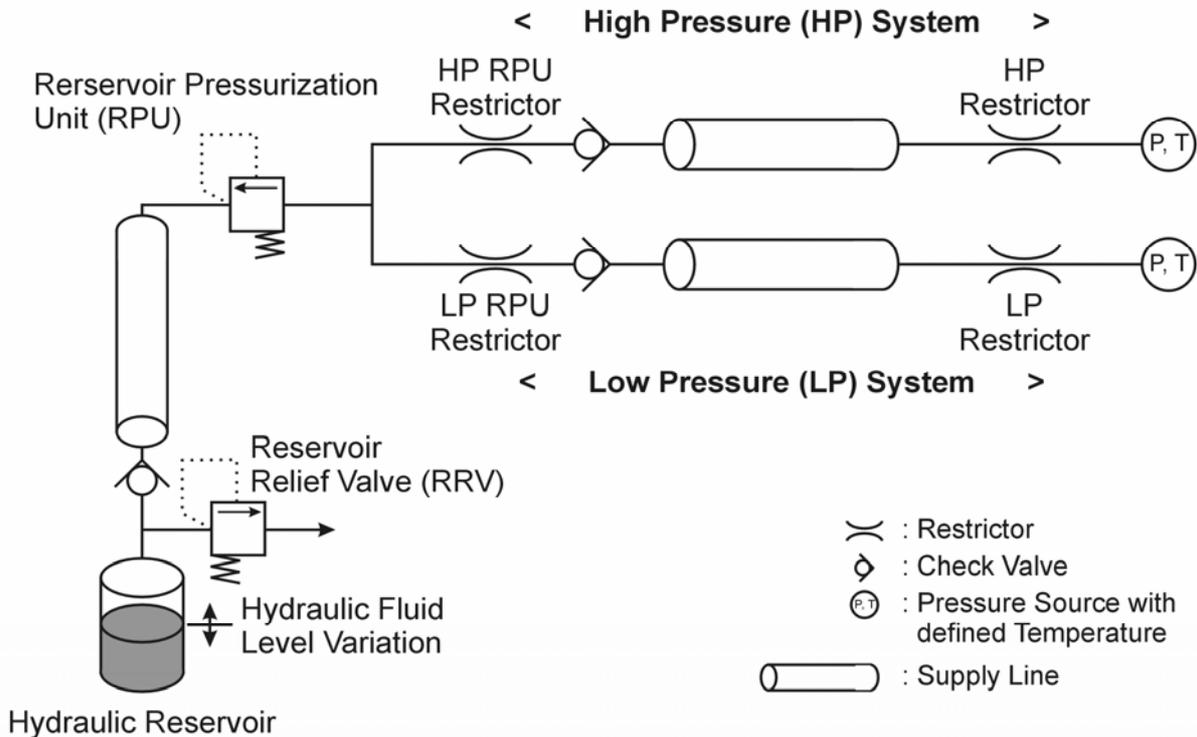
**Figure 1** Simulation system
