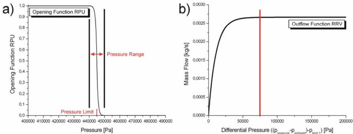
**Figure 2** a) The opening function of the reservoir pressurization unit (RPU) (see Figure 1).
