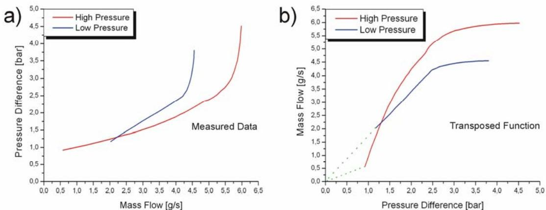
**Figure 3** a) The measured characteristic maps of the used RPU HP (—) and LP restrictors (—) (see Figure 1).
