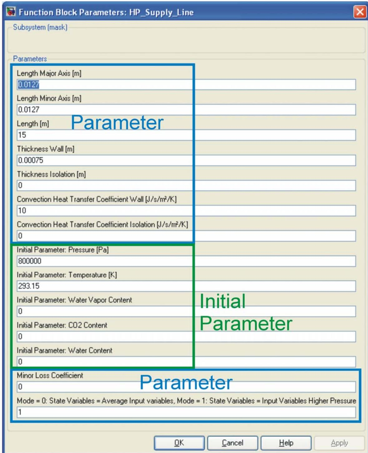
Figure 4 Input mask of the high pressure supply line.
