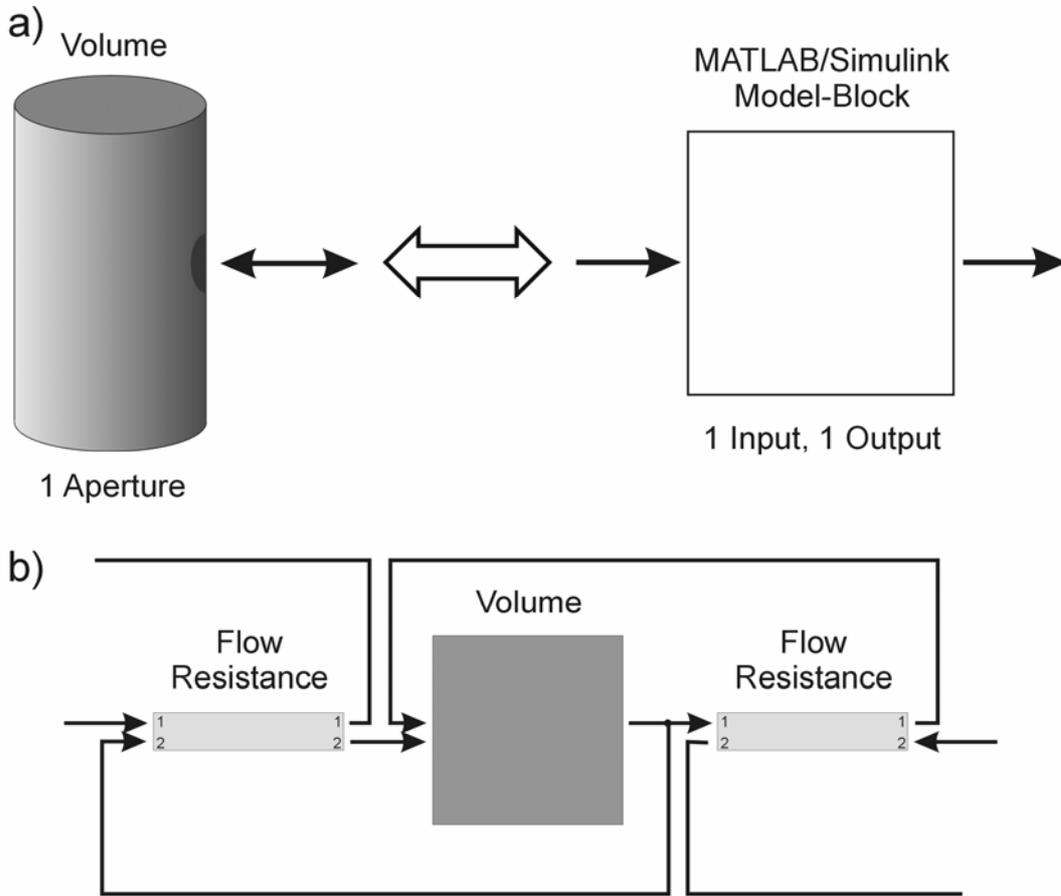
**Figure 5** a) Differentiation between a real component and a MATLAB/Simulink model-block.
