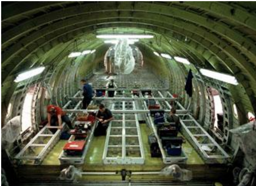
Fig. 3.17 Freighter Conversion of an A300 ( EADS 2009 )
