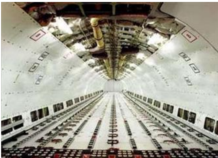
Fig. 3.16 Freighter Cabin of an A300 (EADS 2009)
