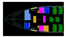
Fig. 1 Cabin layout obtained with Pacelab Cabin tool
