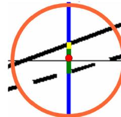
A further increase of the C/G envelope requires a higher  $C_{L,1}/C_{L,2}$ !
