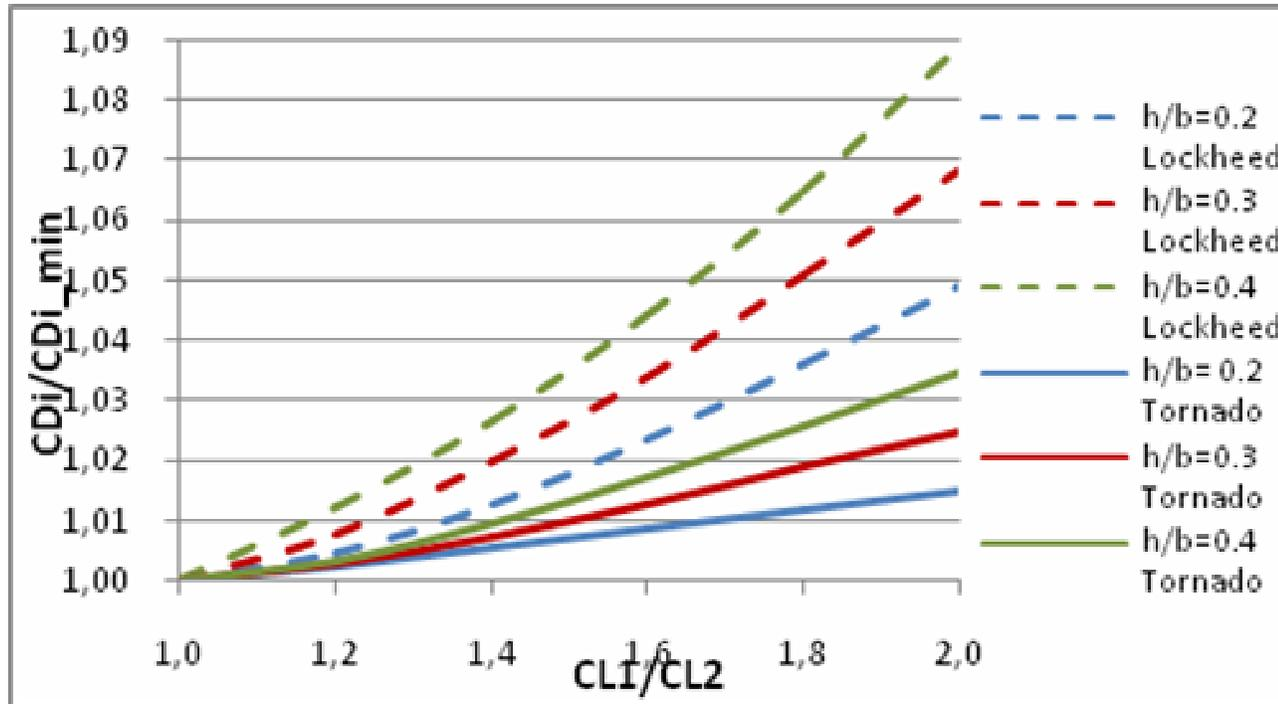
Sensitivity of induced drag to non-optimum lift distributions (Tornado) – Stagger = 0
