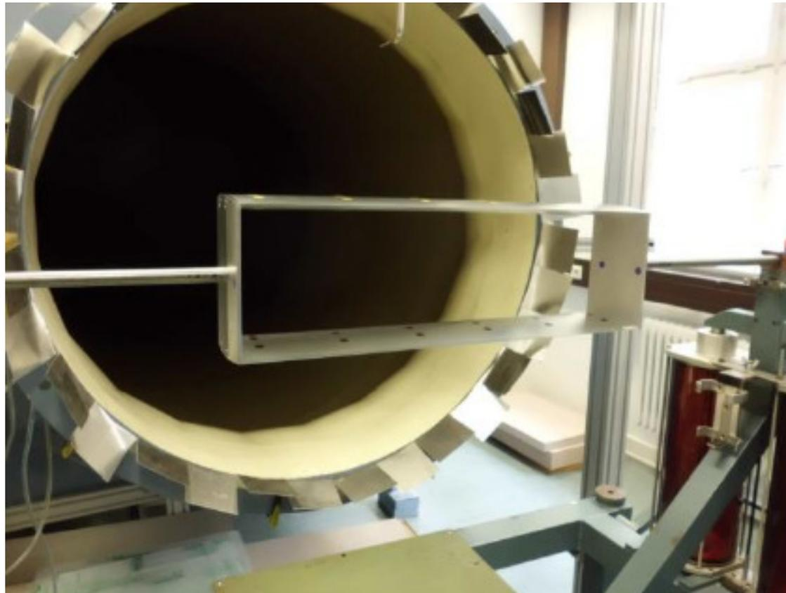
Measurements of induced drag of different box wings in the wind tunnel of HAW Hamburg
