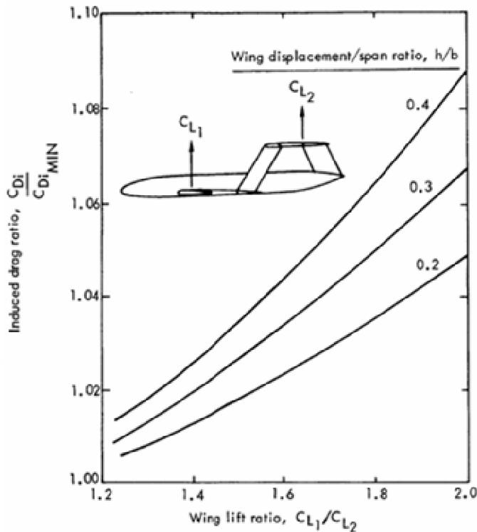
$$\frac{C_{D,i}}{C_{D,i,min}} = \frac{2(x^2 + 1)}{(x + 1)^2} \quad \text{with} \quad x = \frac{C_{L,1}}{C_{L,2}}$$
