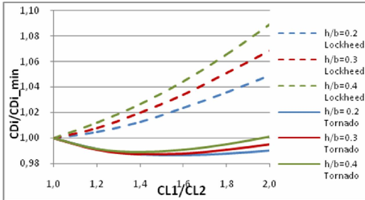
Sensitivity of induced drag to non-optimum lift distributions (Tornado) – Stagger = -0.5b
