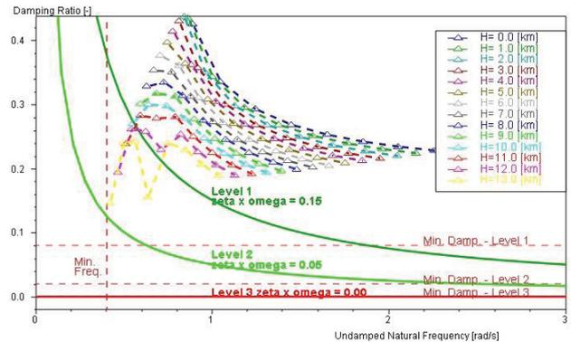
FIG. 14 Dutch Roll mode, 0 m ... 14000 m, 100 m/s ... 240 m/s
