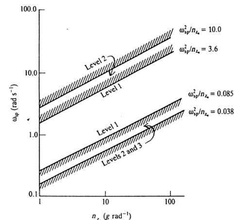
FIG. 11 Chart of the CAP Flight Quality Level Definition, Flight Phase Category B [7]
