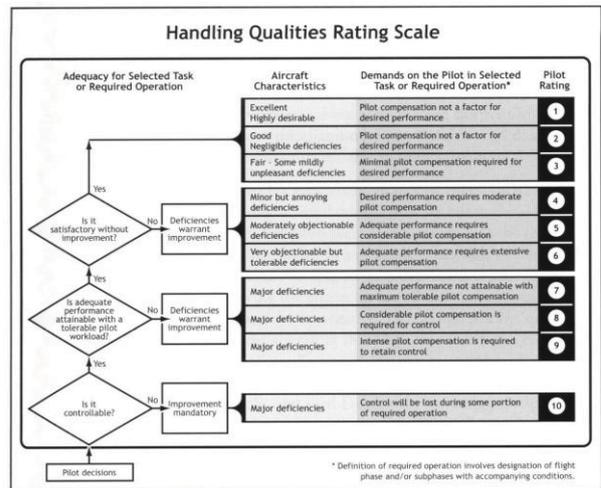
FIG. 19 Cooper-Harper Handling Qualities Rating Scale (www.nasa.gov)
