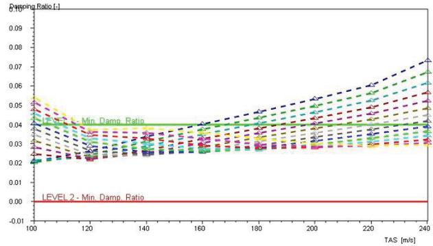
FIG. 13 Phugoid mode, 0 m ... 14000 m, 100 m/s ... 240 m/s
