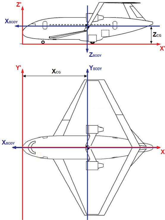
FIG. 4 Reference frames of the box wing aircraft [3]
