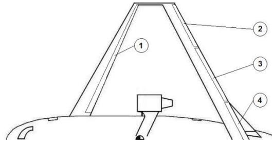
FIG. 3 Control surfaces and high-lift system layout of the box wing aircraft – 1,3: flaps; 2: aileron; 4: elevators [3]
