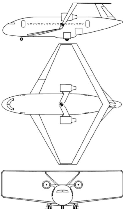
FIG. 2 Three view drawing of the box wing aircraft [2]
