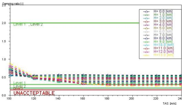
FIG. 12 Short Period mode, 0 m ... 14000m, 100 m/s ... 240 m/s
