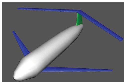
FIG. 16 3D model of the box wing aircraft generated by *Datcom+*
