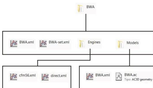
FIG. 15 Files and folders of the box wing aircraft FDM
