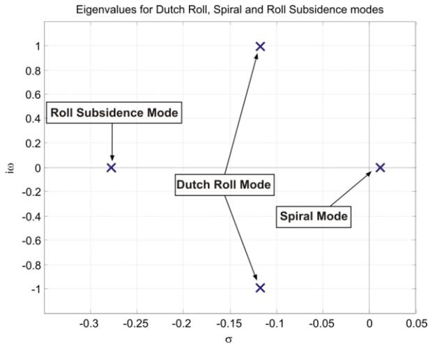
FIG. 10 S-plane for the lateral flight dynamics in cruise conditions
