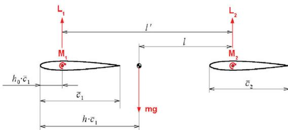
FIG. 5 Forces and moments acting on the box wing aircraft [2]
