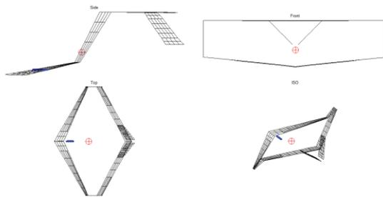
FIG. 7 Meshing of the box wing aircraft in Tornado
