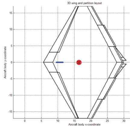
FIG. 8 Top view of the box wing aircraft in Tornado, take-off and landing configuration
