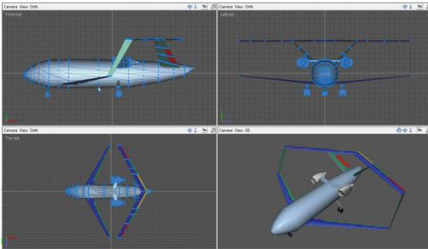
FIG. 17 Final 3D model of the box wing aircraft
