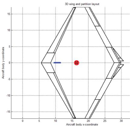
FIG. 6 Top view of the box wing aircraft in Tornado, cruise configuration
