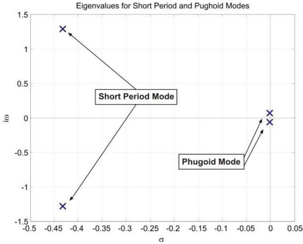
FIG. 9 S-plane for the longitudinal flight dynamics in cruise conditions
