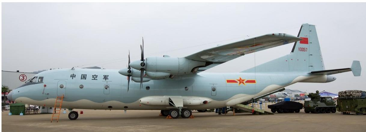
Shaanxi Y-9 multi-purpose transport, developed as a stretched version of the Shaanxi Y-8 with greater payload and range.
