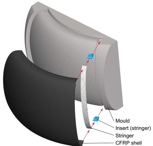
FIG 10. Assembly of the cover shells
