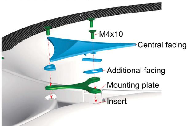
FIG 12. Cell connector between three cells
