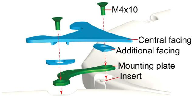
FIG 11. Cell connector between two cells
