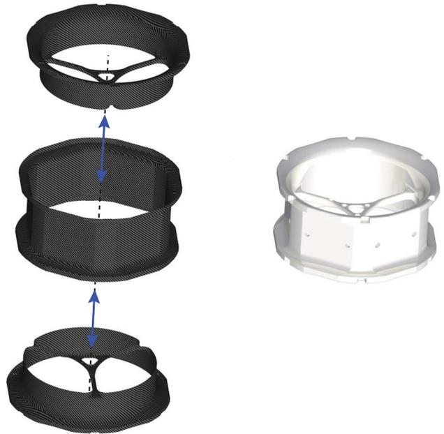
FIG 9. CFRP shell around foam core
