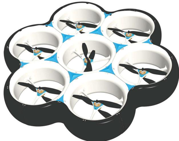
FIG 2. CellDrone made from seven cells
