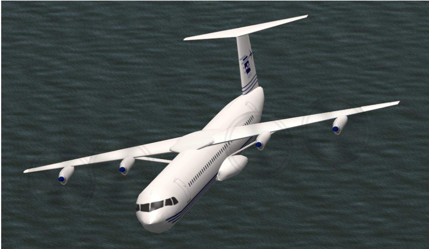
„Smart Turboprop“ with Wing Brace (4 Engines)
