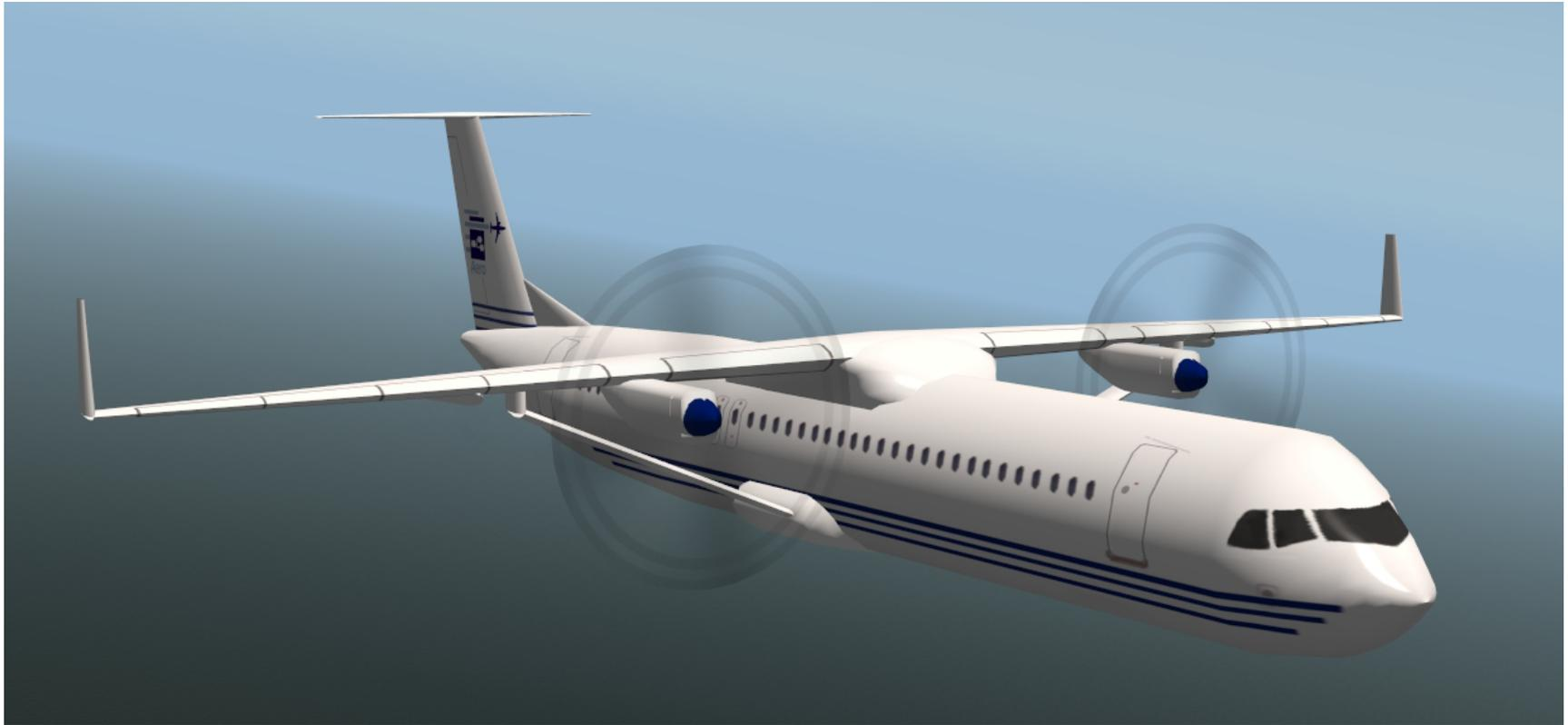
„Smart Turboprop“ with Wing Brace (2 Engines)
