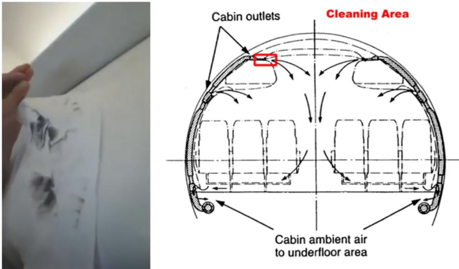
**Figure 21** Left: Cleaning on top of the overhead bins of an Airbus A320 brings to light dirt that is clearly more than dust. The black residue known from the ducts settles also on the bin surface. Picture source: Video: [https://youtu.be/uQfA\\_DiMBS8](https://youtu.be/uQfA_DiMBS8). Right: Airbus A320 cabin cross section with the upper cabin air outlet releasing potentially contaminated air on top of the overhead bins (based on Airbus 1999).
