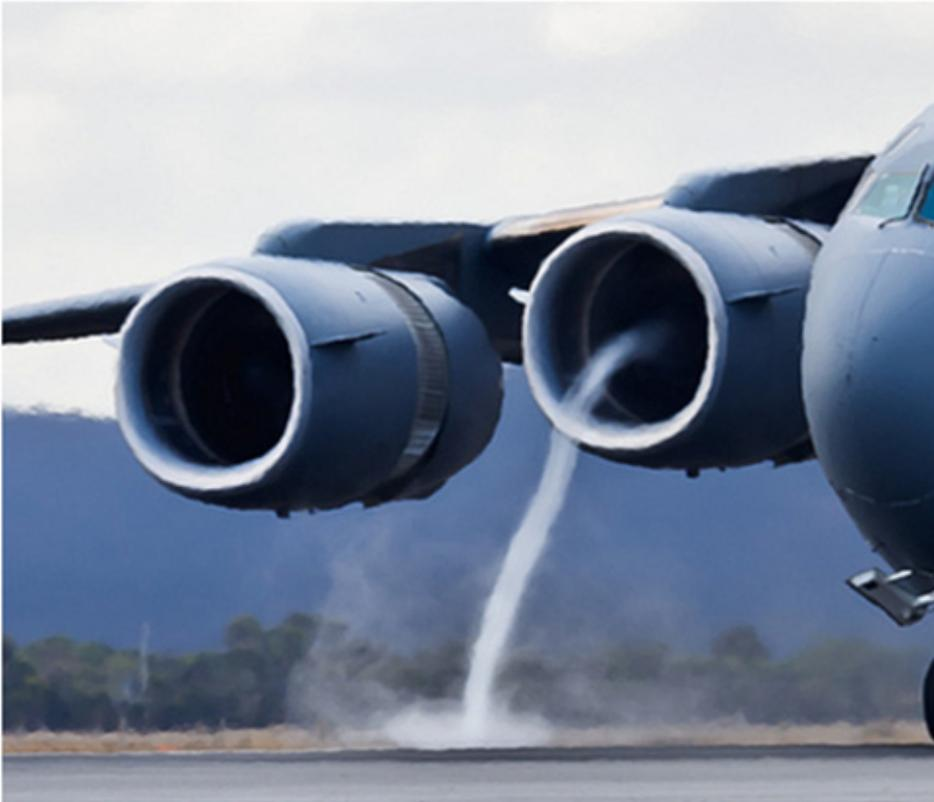
**Figure 32** The ground vortex can also form between the ground and an engine on a high wing (Childs 2017).
