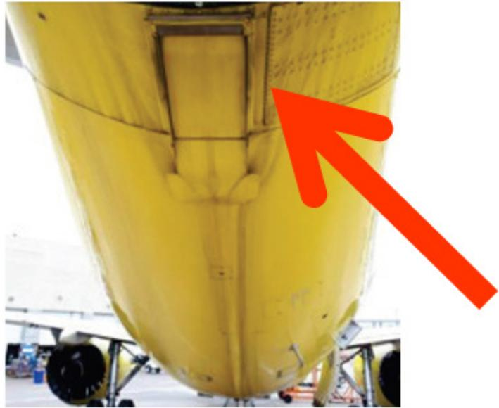
**Figure 24** Air intake of the A320 APU. Source of picture on the right: Airbus 2019.
