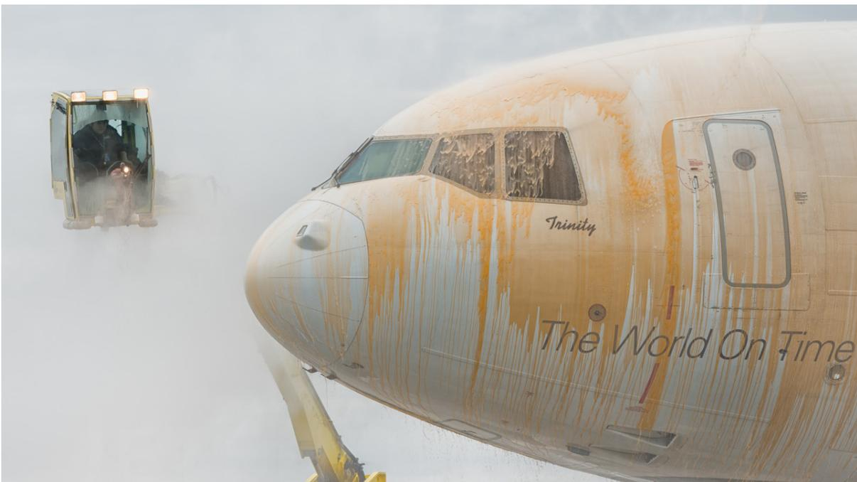
**Figure 27** Leakage of deicing fluid (Petchenik 2015).
