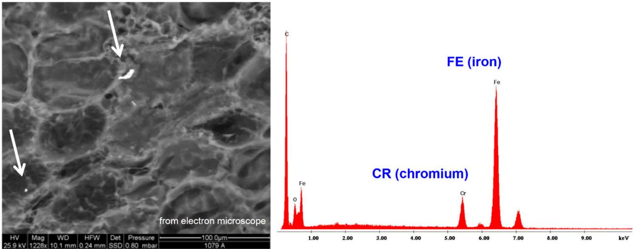
**Figure 4** Analysis 8 of Table I. High-magnification image (1228x) and EDS (Energy-Dispersive X-ray spectroscopy) spectrum of 10-micron and 1-micron brighter-looking particles composed of Carbon, Iron, Chromium and Oxygen: a stainless-steel composition (Gatti 2019, report written for client).
