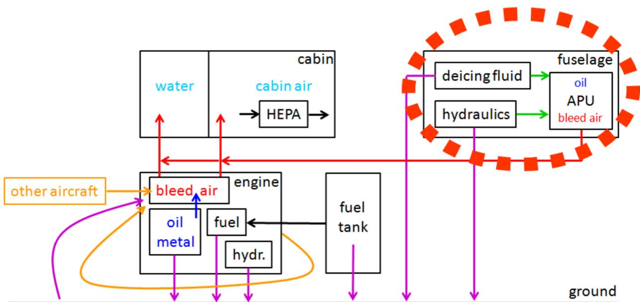
**Figure 22** The route of hydraulic and deicing fluid into the cabin.
