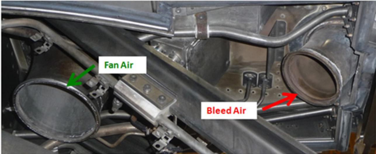
**Figure 12** Bleed air duct with brown stain compared to a clean fan air duct on an Airbus A320.
