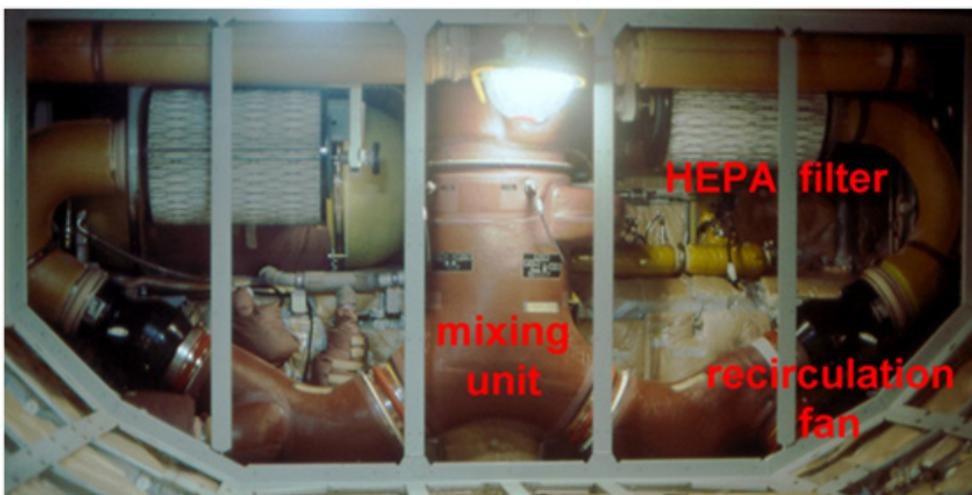
**Figure 33** The main component of the Airbus A320 recirculation system. View from the forward cargo compartment looking aft. The wall panels in the cargo compartment are not installed. The support frames for the wall panels are visible. Two HEPA filters and two recirculation fans are installed symmetrically.
