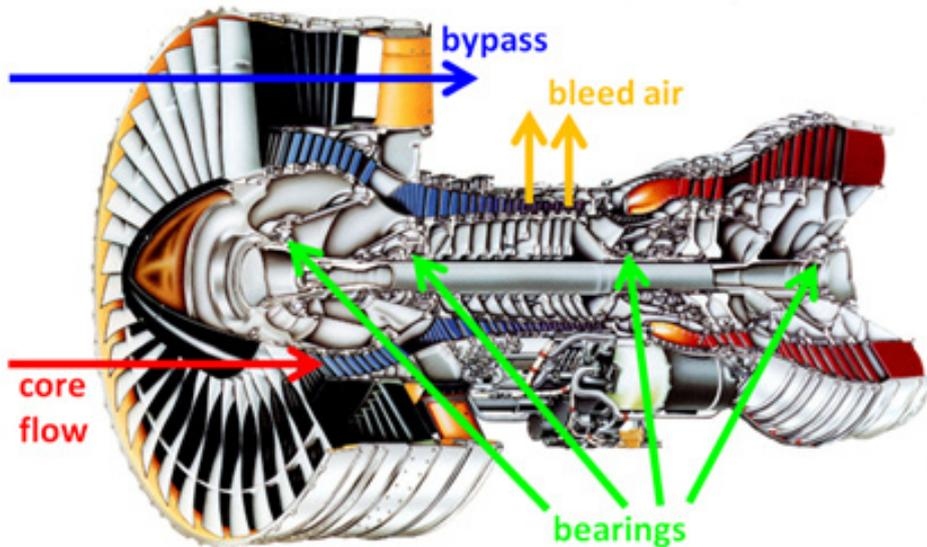
**Figure 2** Engine bearings and bleed air (based on P&W 2014).
