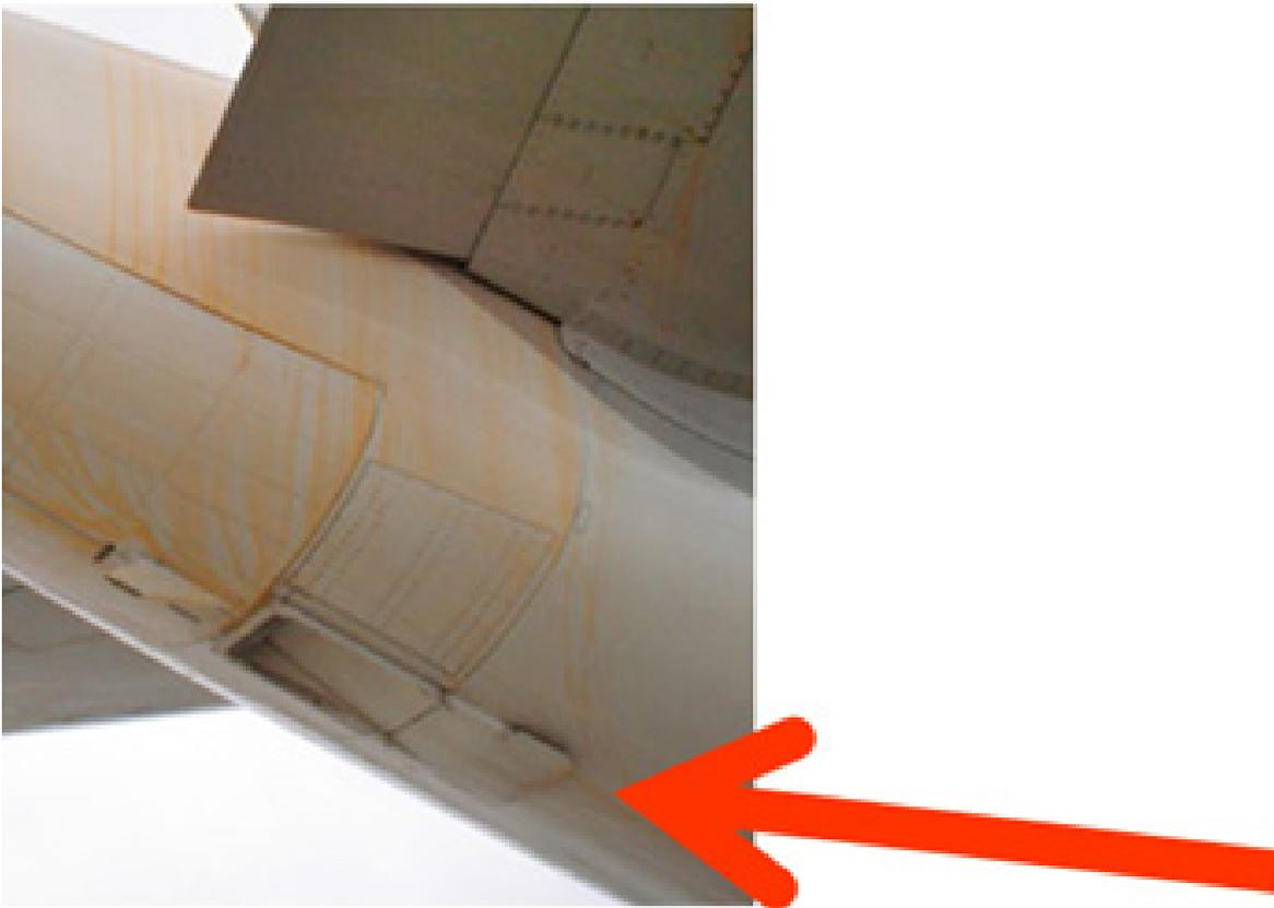
Figure 28 Leakage of deicing fluid on the lower side of the fuselage (Vera-Barcelo 2013).
