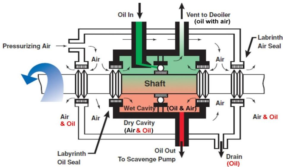
**Figure 3** Lubrication and sealing of engine bearings (based on Exxon 2017).
