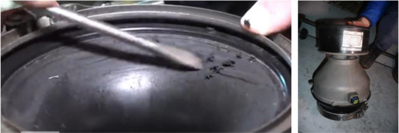
**Figure 34** The recirculation fan of an Airbus A320 is covered by an oily black soft substance that can be scraped off with a screw driver. Picture source: Video: <https://bit.ly/2YXcl3a> (English subtitles available). A disassembled recirculation fan is shown on the right.
