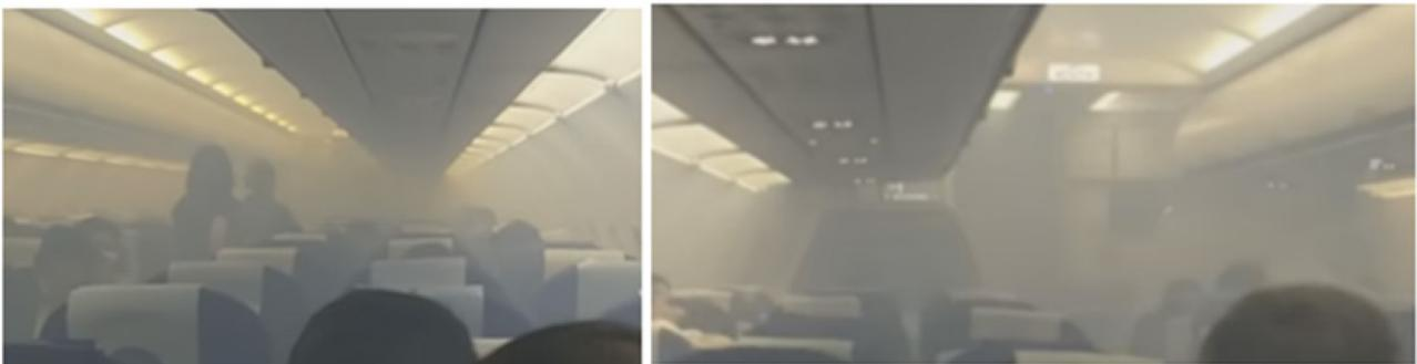
**Figure 7** 2018-12-10, Indigo flight 6E-237, Airbus A320neo, Jaipur to Kolkata, India. The smoke was traced down to the engines (PW1127). This and more: AvHerald 2018. Cause: Leakage of oil from the engine (Telegraph 2018). Picture source: Video: [https://youtu.be/TO\\_FZ3L4yus](https://youtu.be/TO_FZ3L4yus).
