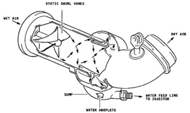
**Figure 14** Engine oil residue accumulates in water extractor. The schematic on the right is from Airbus 1999.
