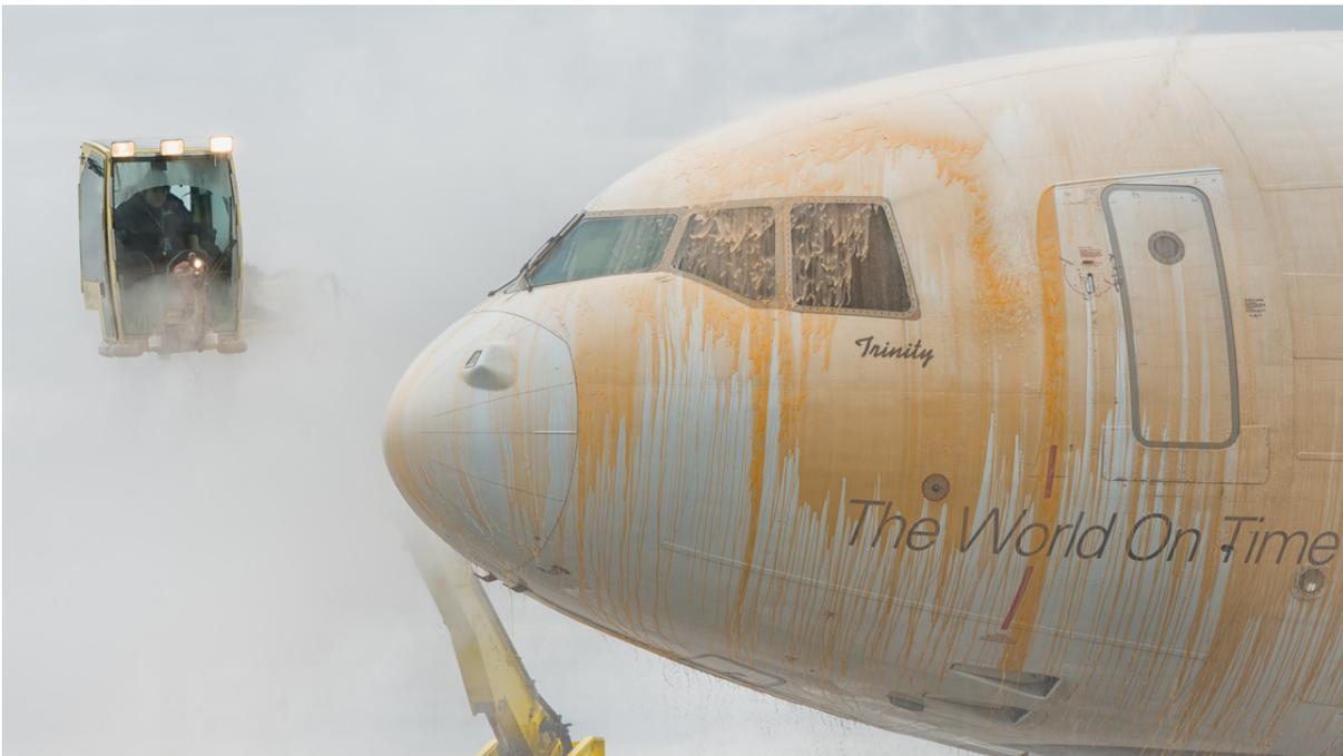
**Figure 27** Leakage of deicing fluid (Petchenik 2015).
