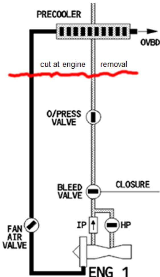
**Figure 11** Fan air and bleed air taken off a jet engine. The red line indicates where the fan air duct and the bleed air duct are separated, when the engine is taken off. The diagram is a simplification based on a diagram explaining the pneumatic system (ATA 36) in the Airbus A320 FCOM.
