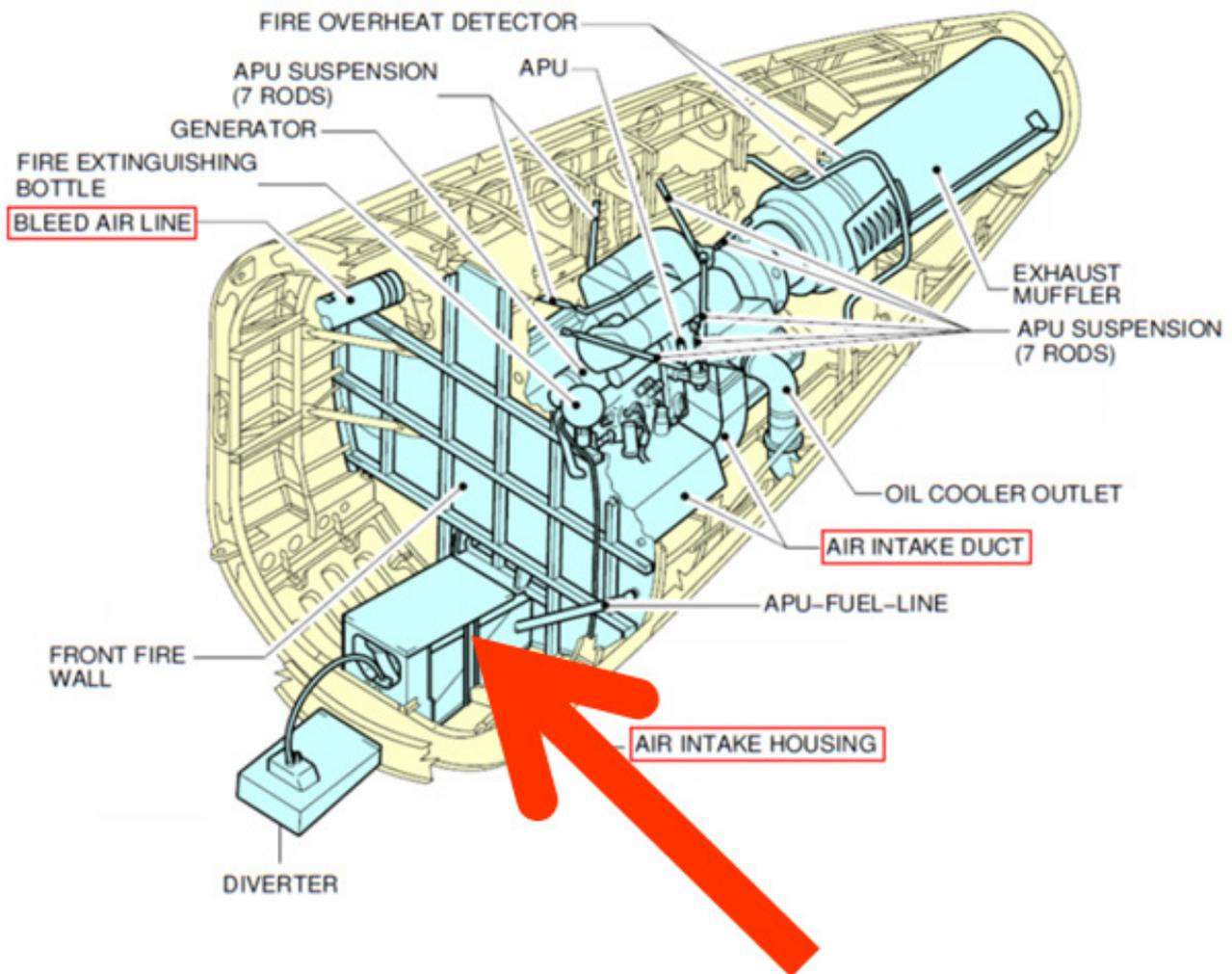
**Figure 23** APU air intake (Airbus 2020).
