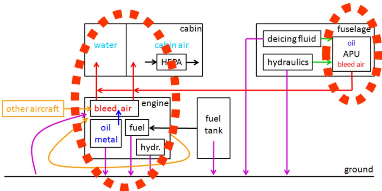
**Figure 5** The route of engine oil into the cabin.
