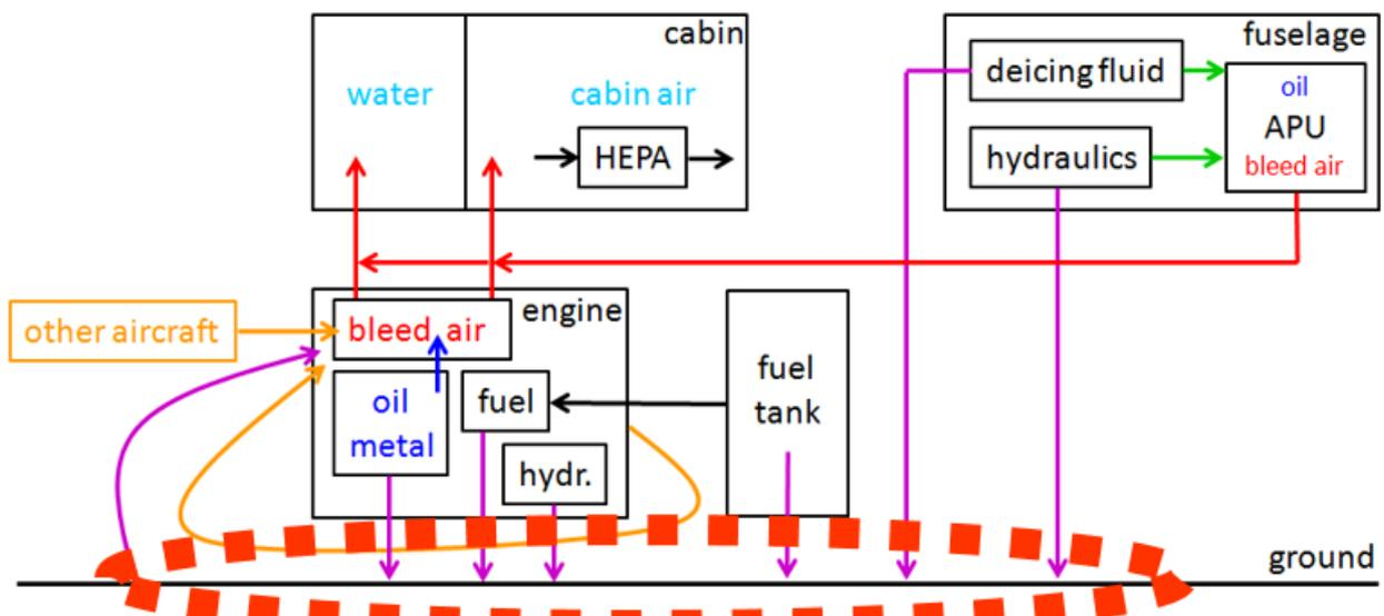
Figure 29 The route of fluids down to the ground and back into the engine.
