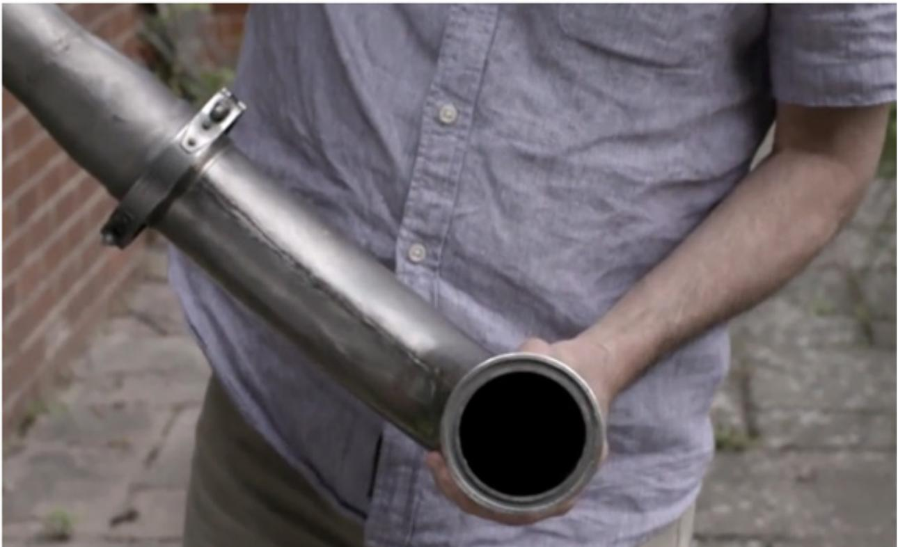
**Figure 13** Engine oil colors bleed air duct black. Picture source: Video: <https://vimeo.com/groups/617439/videos/345959025>.
