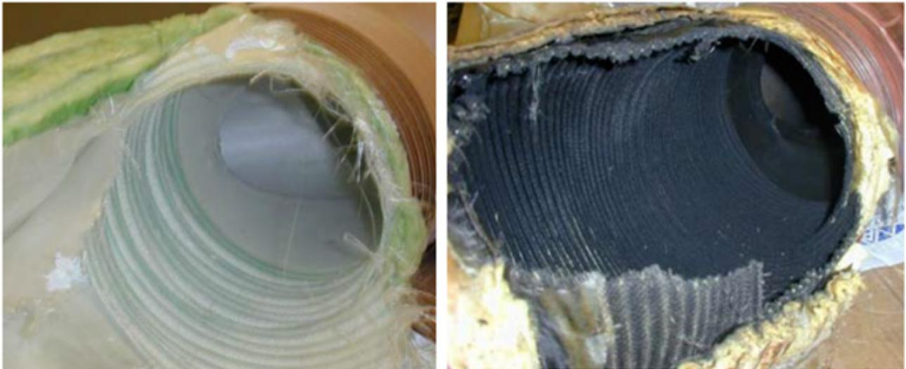
Figure 16 Left: Unused cabin air duct. Right: Used cabin air duct on a BAe 146 passenger aircraft (CAA 2004).
