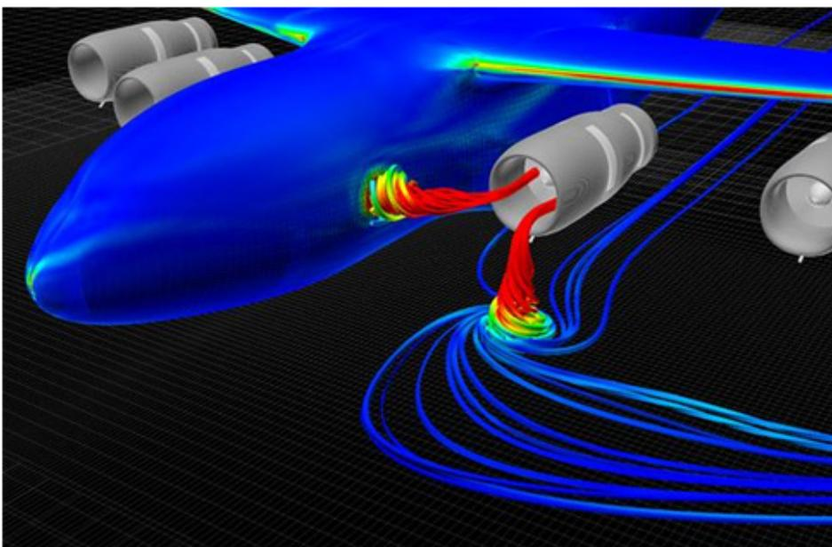
**Figure 31** Simulation of two intake vortices, one of them as a ground vortex. The rotation of the vortex is visible. Picture source: <https://perma.cc/VH99-87XS>.
