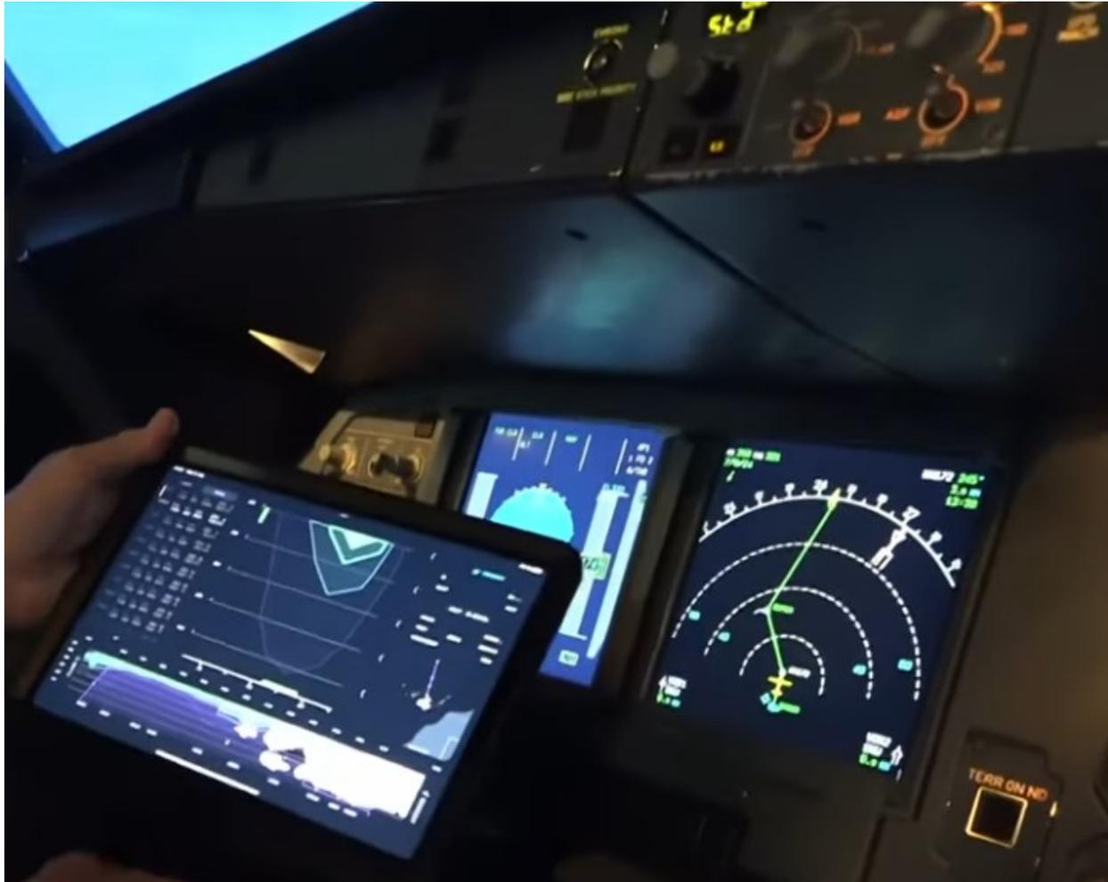
Use of the Electronic Flight Bag (EFB) on a tablet in an Airbus A320 cockpit.
