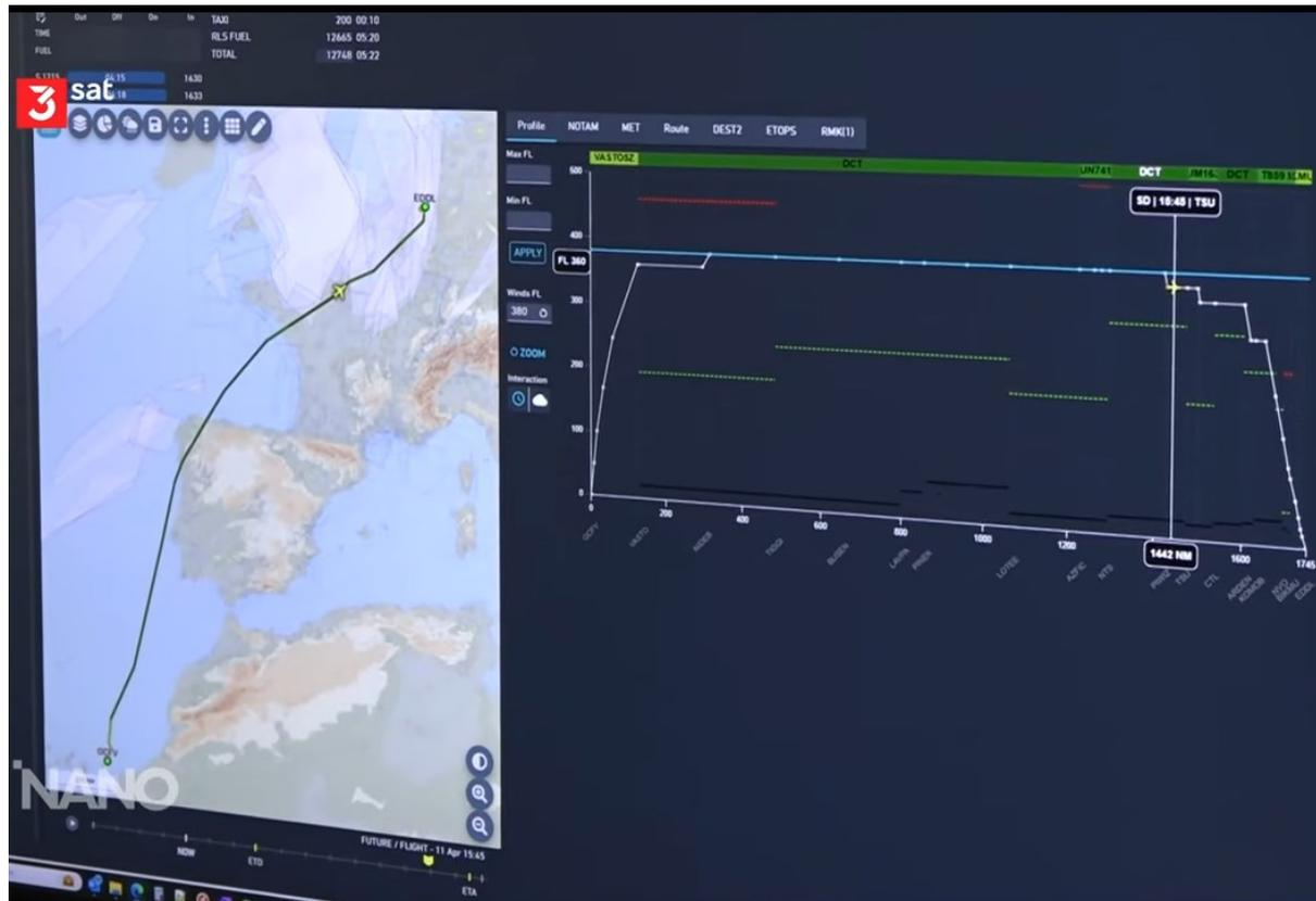
FlightKeys flight planning system "5D" with new features for contrail avoidance.
