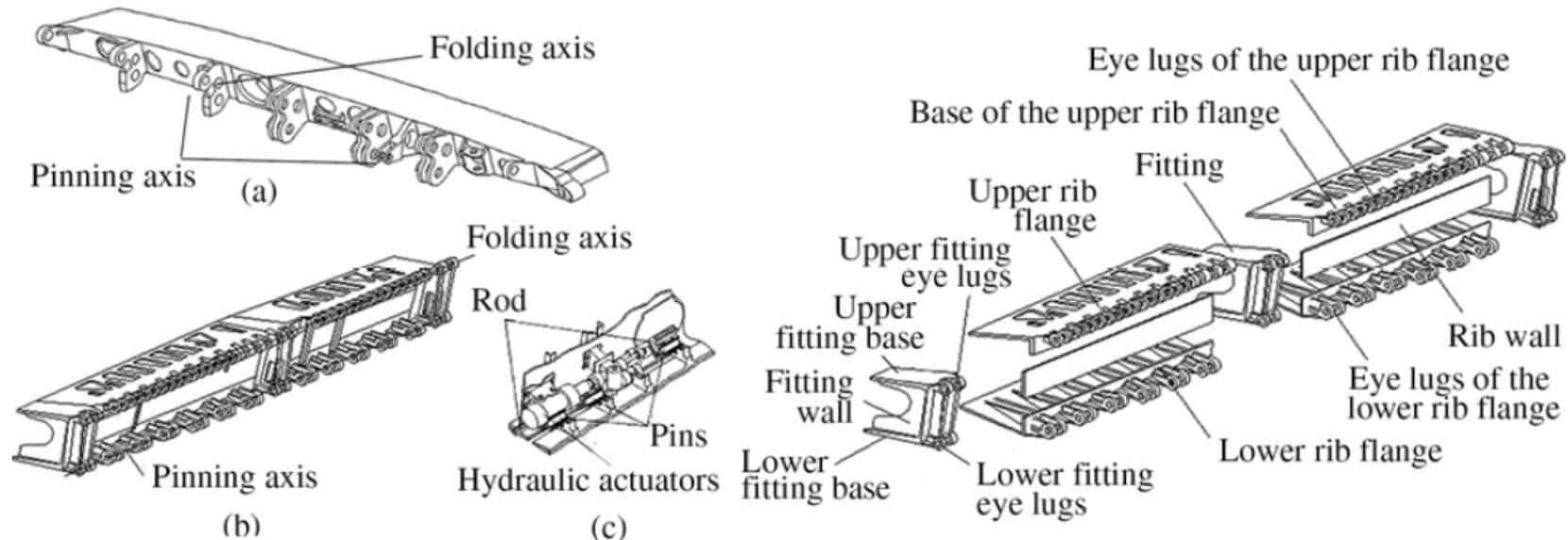
The wing bending moment is taken up by panels. The fold is designed with eye-lugs. They merge within each other like two combs. The upper eye-lugs are the folding axis, the lower eye-lugs are the pinning axis. a) MIG-29K, b) Su-33, c) actuator in the folding mechanism. (Yarygina 2012b)
