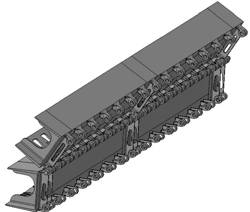
The folding wing of the **Su-33**. The upper eye-lugs are the folding axis, the lower eye-lugs are the pinning axis. An actuation arm is visible. Hydraulics and electrics are routed through the fold to supply the outer part of the wing. Left: **Popov 2011**. Right: **Yarygina 2012c**.
