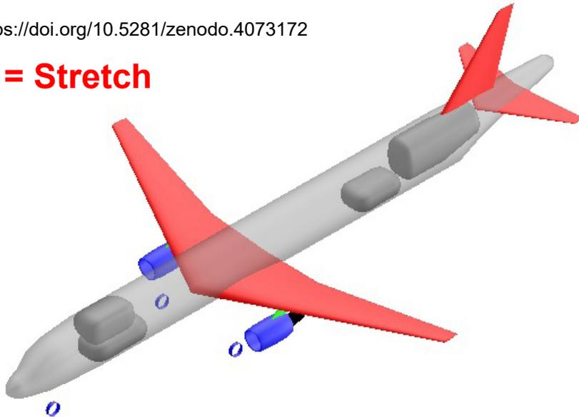
Details of the tanks for the A321-HS
