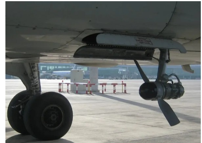
Ram Air Turbine
