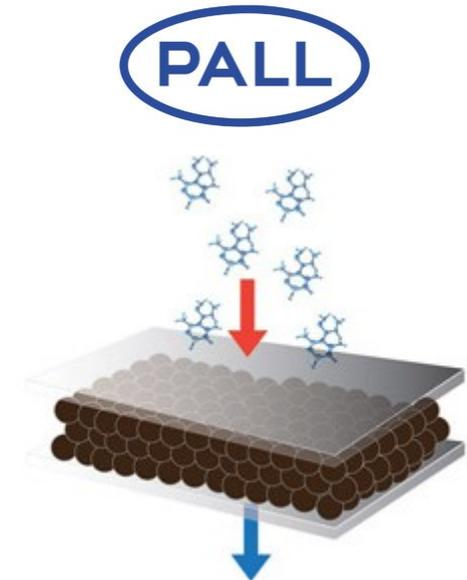
Schematic of carbon filter
