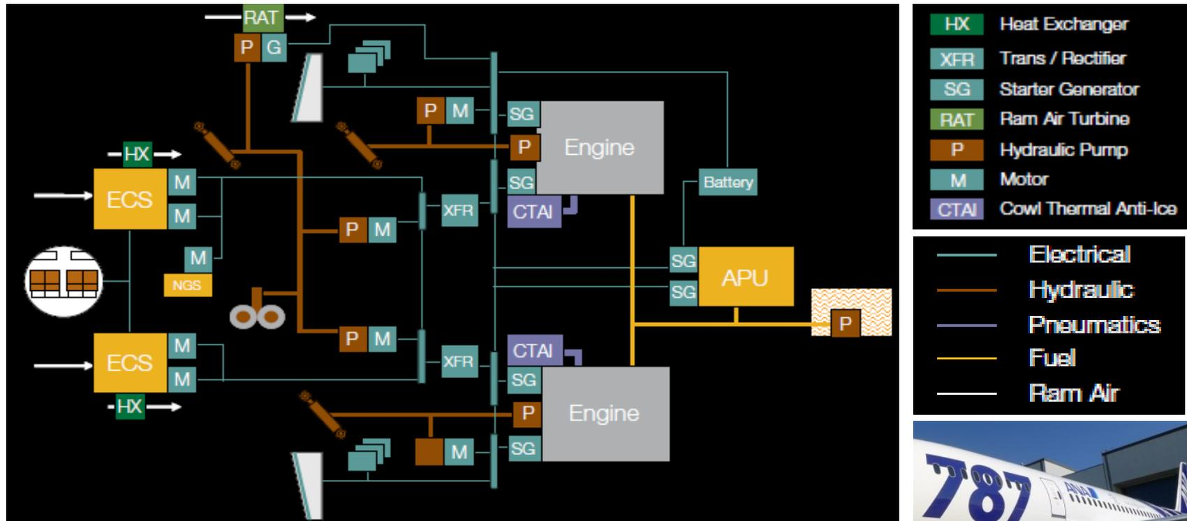
The "Pack" of the B787's Environmental Control System (ECS) is powered by electric motors (M) to compress ambient air up to cabin pressure and to push the air through the heat exchangers (HX) for cooling. The power for the electric motors is produced by generators (SG) connected to the aircraft's engine and APU. After compression and cooling the air is delivered to the cabin.
