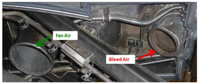
Figure 12 Bleed air duct with brown stain compared to a clean fain air duct on an Airbus A320.
