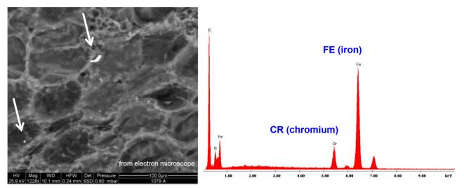
Figure 4 Analysis 8 of Table I. High-magnification image (1228x) and EDS (Energy-Dispersive X-ray spectroscopy) spectrum of 10-micron and 1-micron brighter-looking particles composed of Carbon, Iron, Chromium and Oxygen: a stainless-steel composition (Gatti 2019, report written for client).
