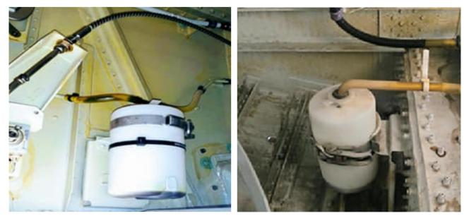
Figure 25 Forward (left) and aft (right) collector tank of the A320 seal drain system (Mekanikong 2019a and 2019b).
