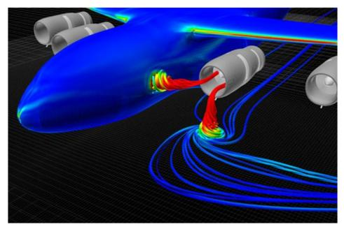
Figure 31 Simulation of two intake vortices, one of them as a ground vortex. The rotation of the vortex is visible. Picture source: <u>https://perma.cc/VH99-87XS</u>.
