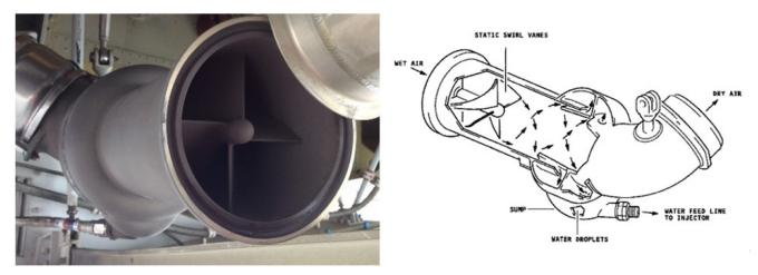
Figure 14 Engine oil residue accumulates in water extractor. The schematic on the right is from Airbus 1999.
