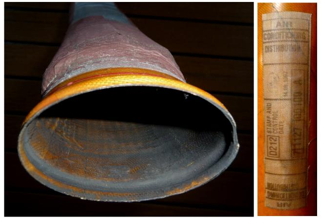
Figure 20 View into the riser duct where it was separated at the cabin floor. It is covered inside by black residue.
