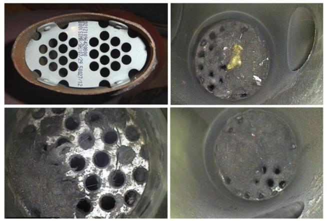
Figure 18 Top left: Clean flow limiter in an air conditioning duct on an Airbus A320 (here in a dead-end duct section) compared to flow limiters clogged from pyrolyzed engine oil in ducts of the air conditioning system of Boeing 757 aircraft (Hansen 2019).
