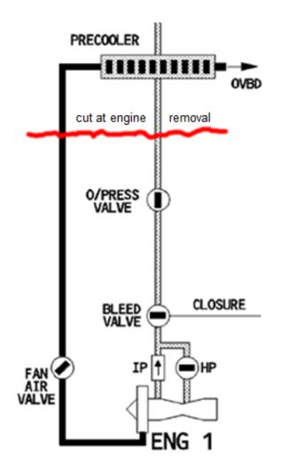
Figure 11 Fan air and bleed air taken off a jet engine. The red line indicates where the fan air duct and the bleed air duct are separated, when the engine is taken off. The diagram is a simplification based on a diagram explaining the pneumatic system (ATA 36) in the Airbus A320 FCOM.
