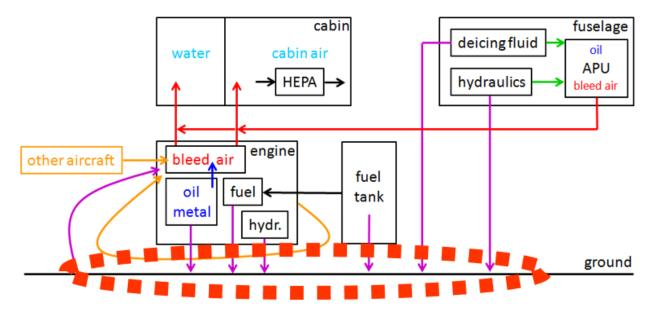
Figure 29 The route of fluids down to the ground and back into the engine.
