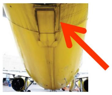
Figure 24 Air intake of the A320 APU. Source of picture on the right: Airbus 2019.
