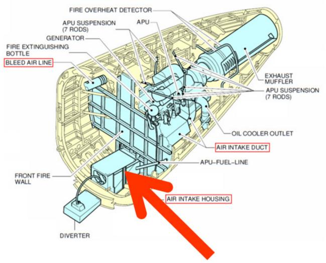
Figure 23 APU air intake (Airbus 2020).
