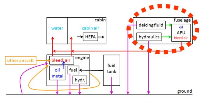
Figure 22 The route of hydraulic and deicing fluid into the cabin.
