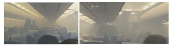
Figure 7 2018-12-10, Indigo flight 6E-237, Airbus A320neo, Jaipur to Kolkata, India. The smoke was traced down to the engines (PW1127). This and more: AvHerald 2018. Cause: Leakage of oil from the engine (Telegraph 2018). Picture source: Video: <u>https://youtu.be/TO\_FZ3L4yus</u>.
