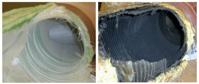
Figure 16 Left: Unused cabin air duct. Right: Used cabin air duct on a BAe 146 passenger aircraft (CAA 2004).
