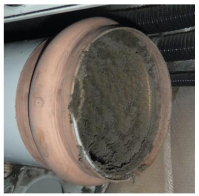
Figure 35 The ambient air inlet in the cargo compartment of the Airbus A320 for cargo compartment heating and ventilation. The inlet is full of moist dust.
