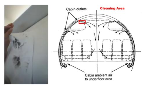
Figure 21 Left: Cleaning on top of the overhead bins of an Airbus A320 brings to light dirt that is clearly more than dust. The black residue known from the ducts settles also on the bin surface. Picture source: Video: <u>https://youtu.be/uQfA DiMBS8</u>. Right: Airbus A320 cabin cross section with the upper cabin air outlet releasing potentially contaminated air on top of the overhead bins (based on Airbus 1999).
