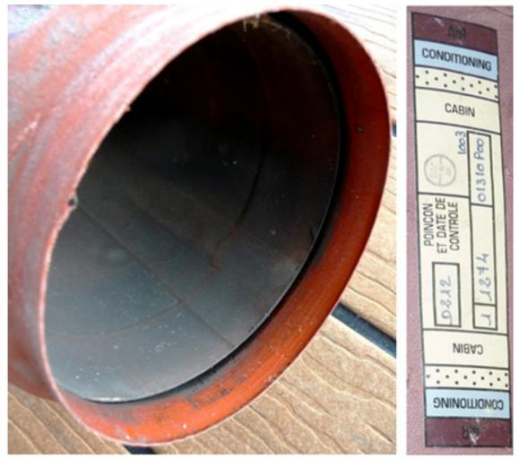
Figure 15 Airbus A320 air conditioning air distribution duct in the cabin.
