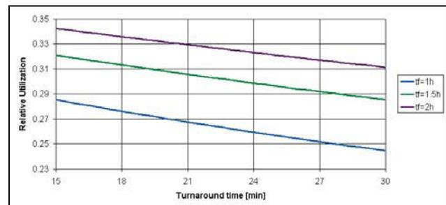
FIG 11. Relative utilization against turnaround time for different flight times  $t_f$
