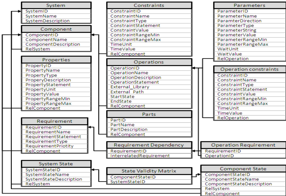
Figure C.6 MAIP-database schema of CAM
