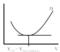
$$\left(\begin{array}{c} L \\ D \end{array}\right)_{\text{max}} = \frac{1}{2\sqrt{C_{D_{0L}}K}}$$
