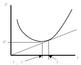
Hence the smallest angle obtained by drawing the tangent line as shown in the figure will give the point where the drag is a minimum, and the corresponding airspeed for the maximum range flight condition.
