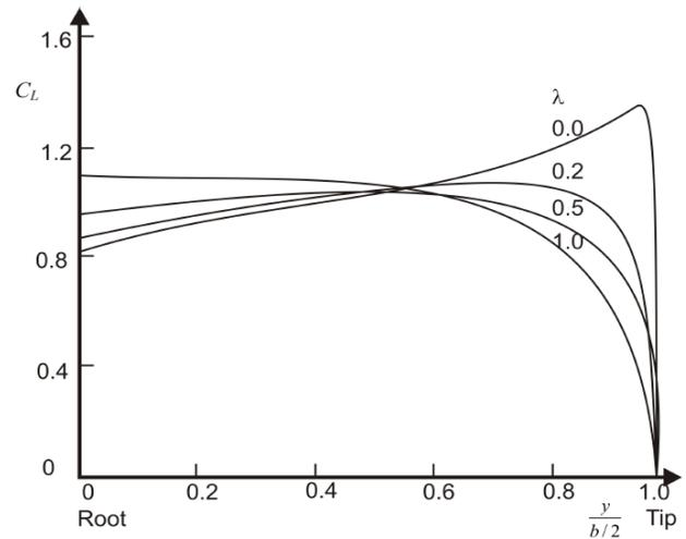
The wing with the taper ratio  $\lambda = 0$  will stall, because it "tries to achieve" a local lift coefficient larger than 1.2 on the wing tip i.e. outboard of 80 % halfspan.
