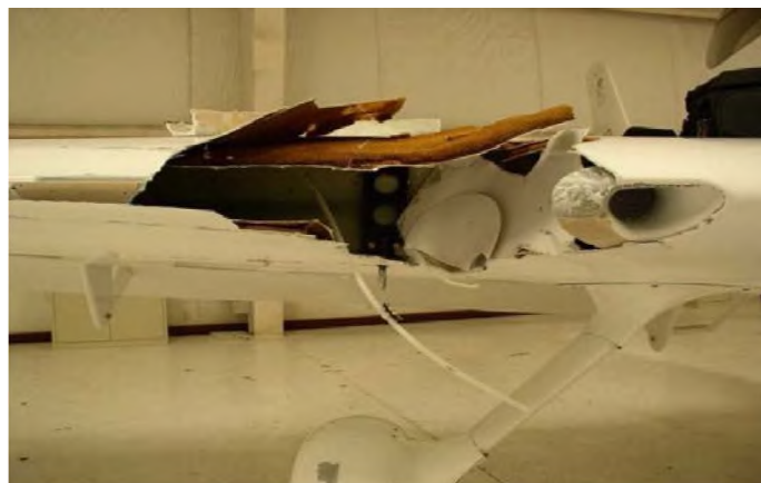
Fig.4. Destruction of leading-edge wing extension in a collision with a foreign object
