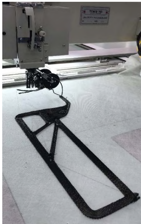
Fig. 7. Sub-preform of the hatch, made on the equipment of Tajima for technology Tailored fiber placement
