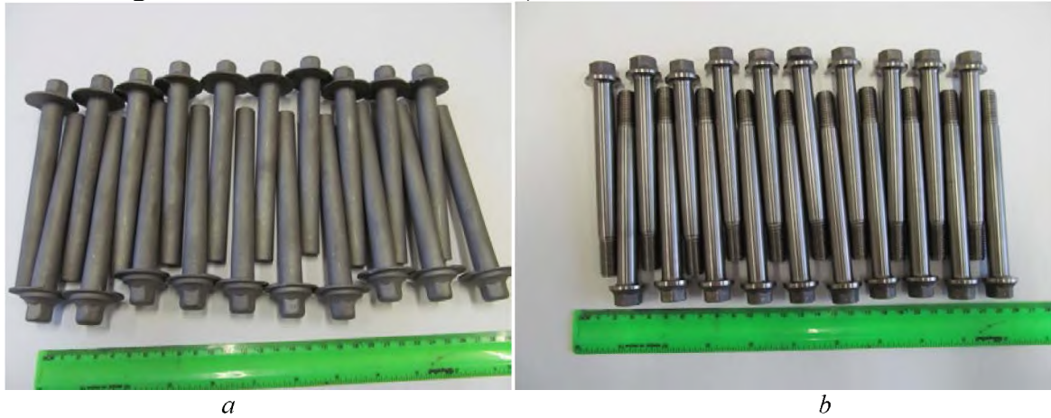
Fig. 7. Titanium screw-bolts from an alloy FT-01: a – after the hot landing heads of bolt; b – finally made.
