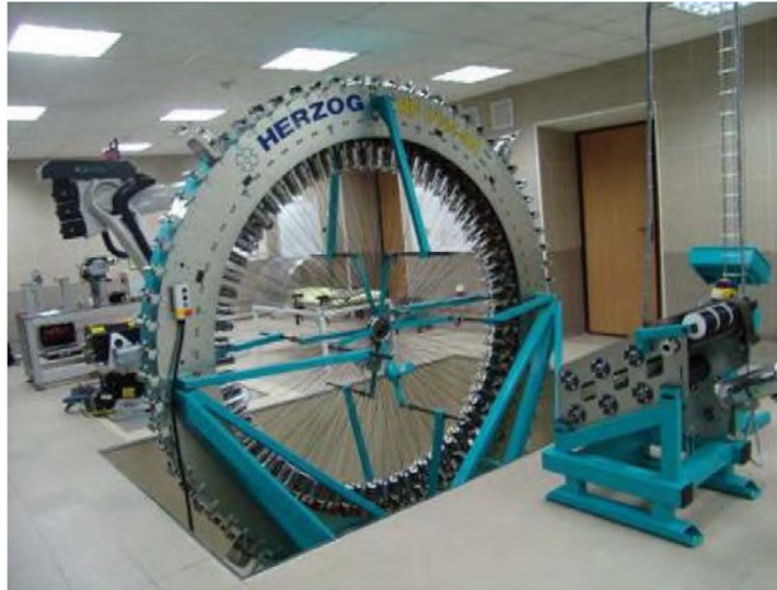
Fig. 10. Robotic complex creation of preforms by the method of radial braiding. Conducting the experimental part.
