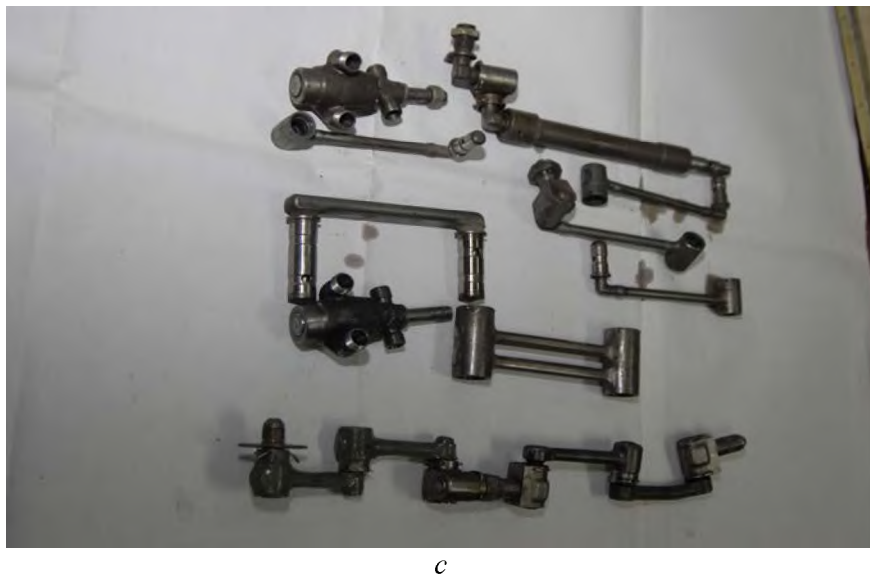
Fig.5. Titanium components wares of hydraulic of airplane: a -hydraulic cylinder; b - stock of hydraulic cylinder; c - joint wiring of TC18
