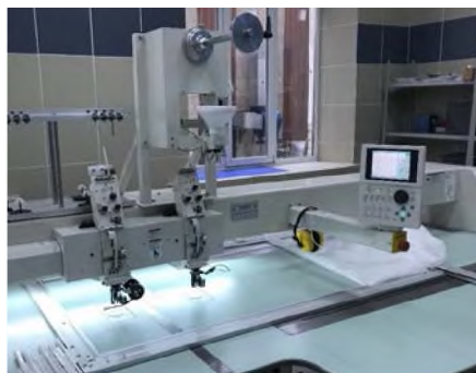
Fig. 1. Specialized Tajima machine for Tailored fiber placement technology
