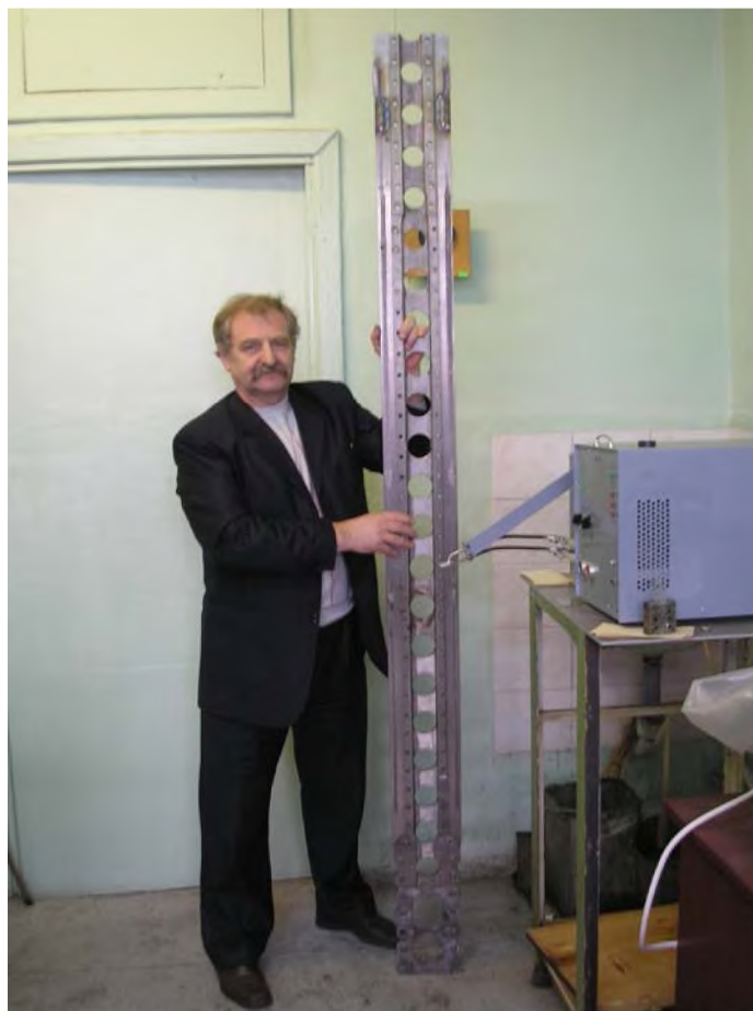
Fig.4. Rail of control system of flap airplane AN 124 "Ruslan" from the alloy of TC18
