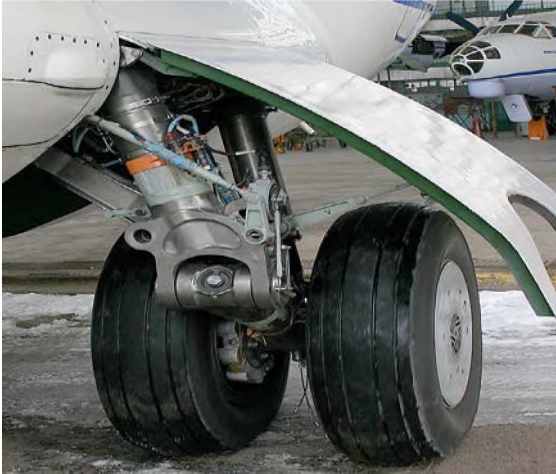
Fig.2 Stand of undercarriage of airplane from the alloy of TC18 (BT 22 or Ti-5-5-5-1-1.5)
