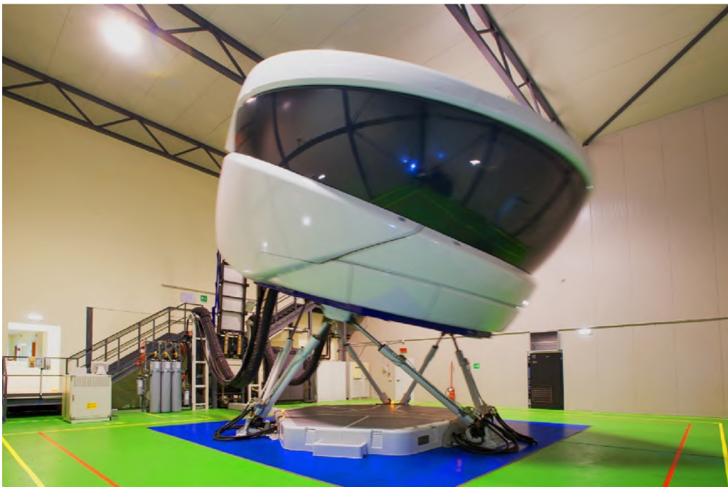
Fig.1. Super Jet international flight simulator FFS 1 installed by L3 CTS.
