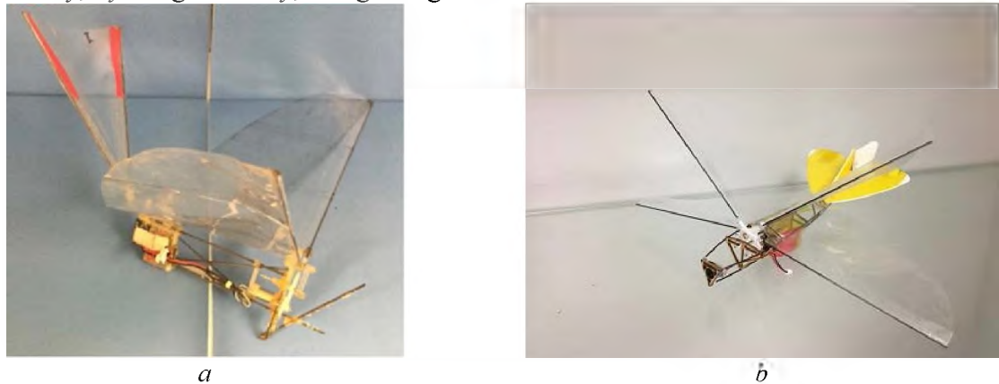
Fig.1. Flapping wing MAVs of PolyU: a – two-wing flapping wing MAV; b – four-wing flapping wing MAV
