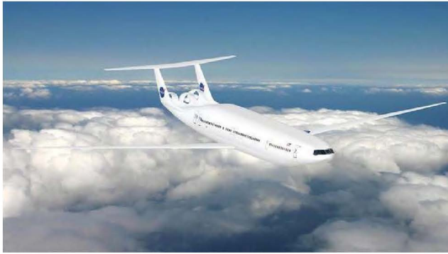
Figure 6: MIT Double-bubble Fuselage with Aft-mounted engines
