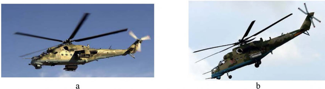
Figure 10: a – Mi-24 landing gear retracted, b – Mi-35 non-retractable landing gear [1,2]
