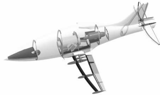
Fig. 6 Structure layout of demonstrator
