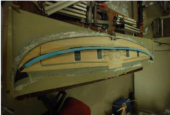
Fig. 8 Molding of the wing
