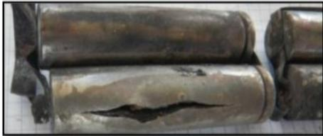
Fire damaged remains of battery pack with a fractured cell
