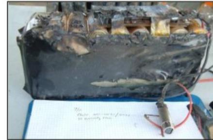
36-cell lithium-ion battery pack with thermal damage.
