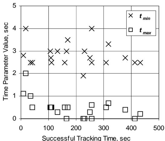
**Figure 14. Effect of Boundary Tracking Time Parameters on Tracking Success.**
