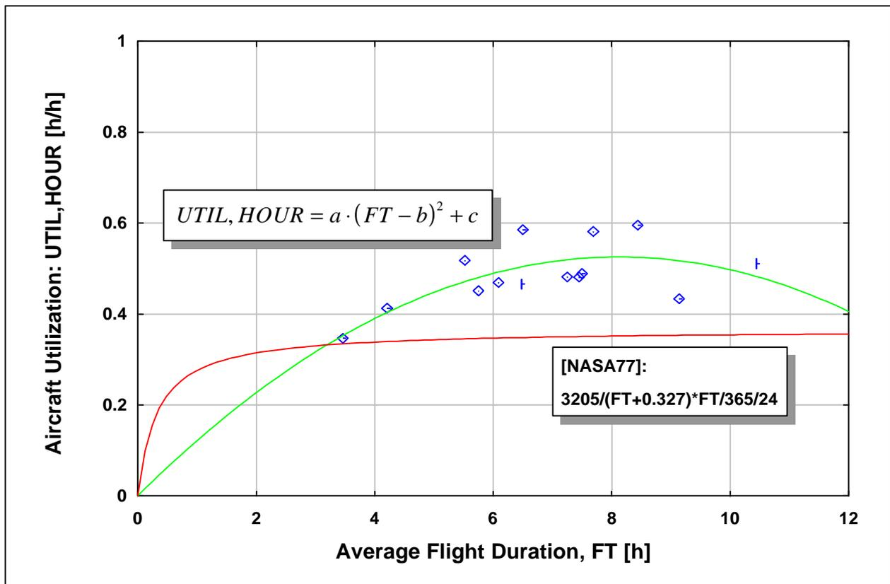
**Fig. 4.2:** Relationship of flight time,  $FT$ , and hourly aircraft utilization,  $UTIL, HOUR$ . Data from A340 fleet [AIRBUS 96] compared with a relationship from [NASA 77] and a correlation of A340 fleet data.
