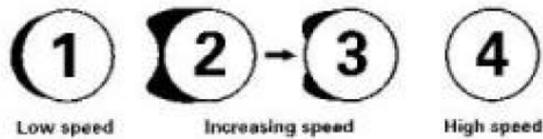
**Figure 6.11** Speed have an effect on ice accretion
