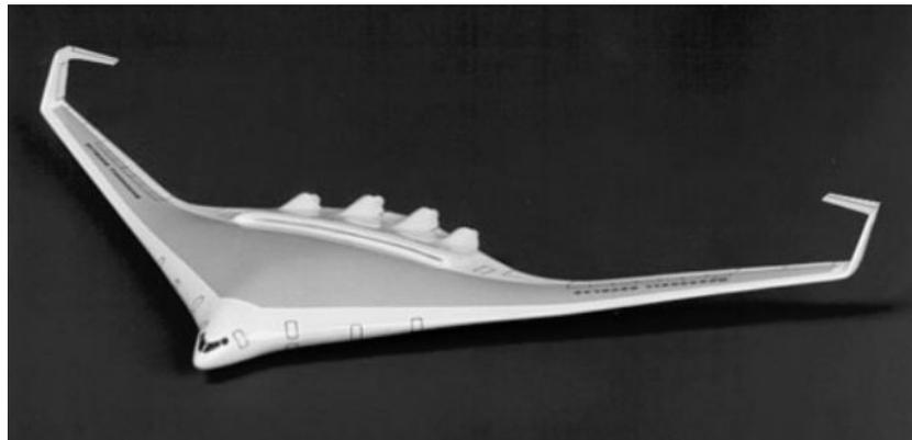
**Figure 2.9 - Blended-wing-body concept with C-wing configuration for enhanced stability and control (Kroo I. , 2005)**
