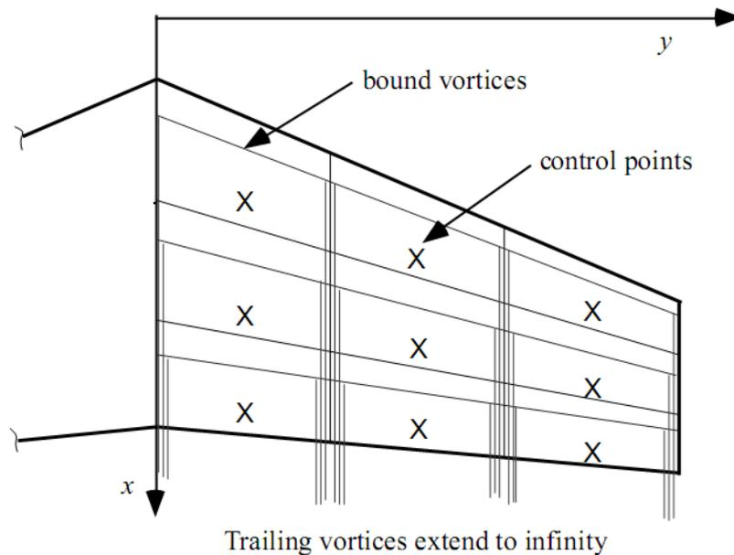
**Figure 4.1 - The horseshoe vortex layout for a vortex lattice method (Mason, 1995)**
