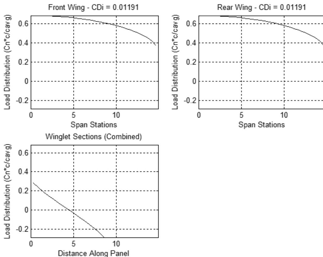
**Figure 4.8 - Computed optimum span load distribution for box-wing aircraft**
