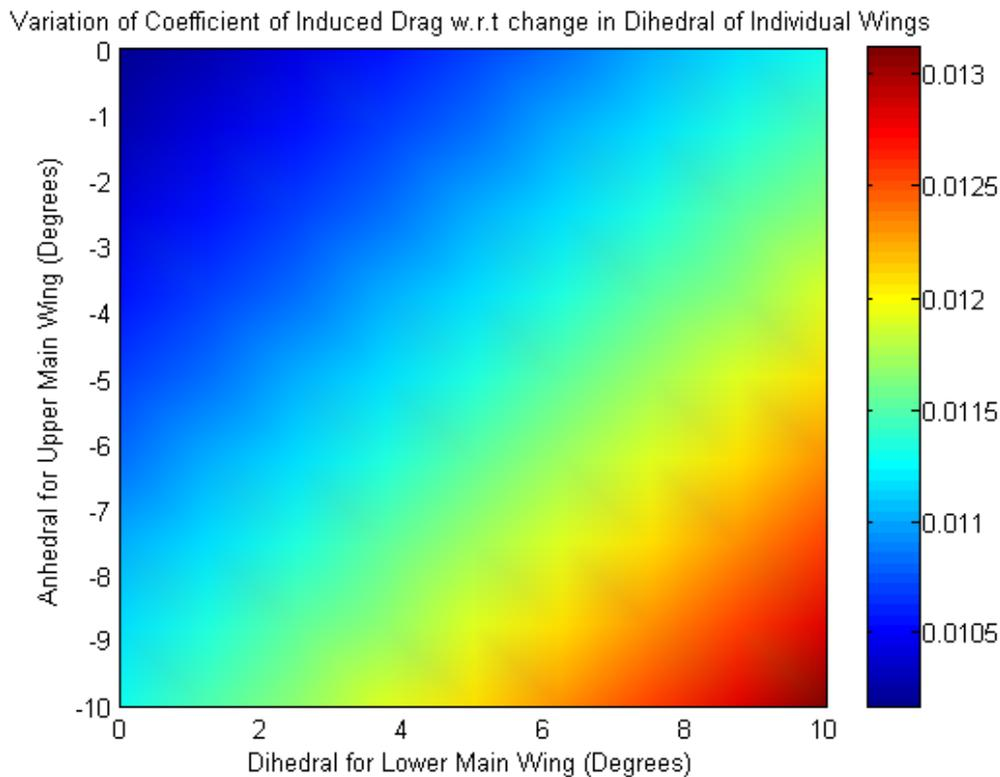
**Figure 4.3 - Variation of coefficient of induced drag with change in dihedral for individual wings**
