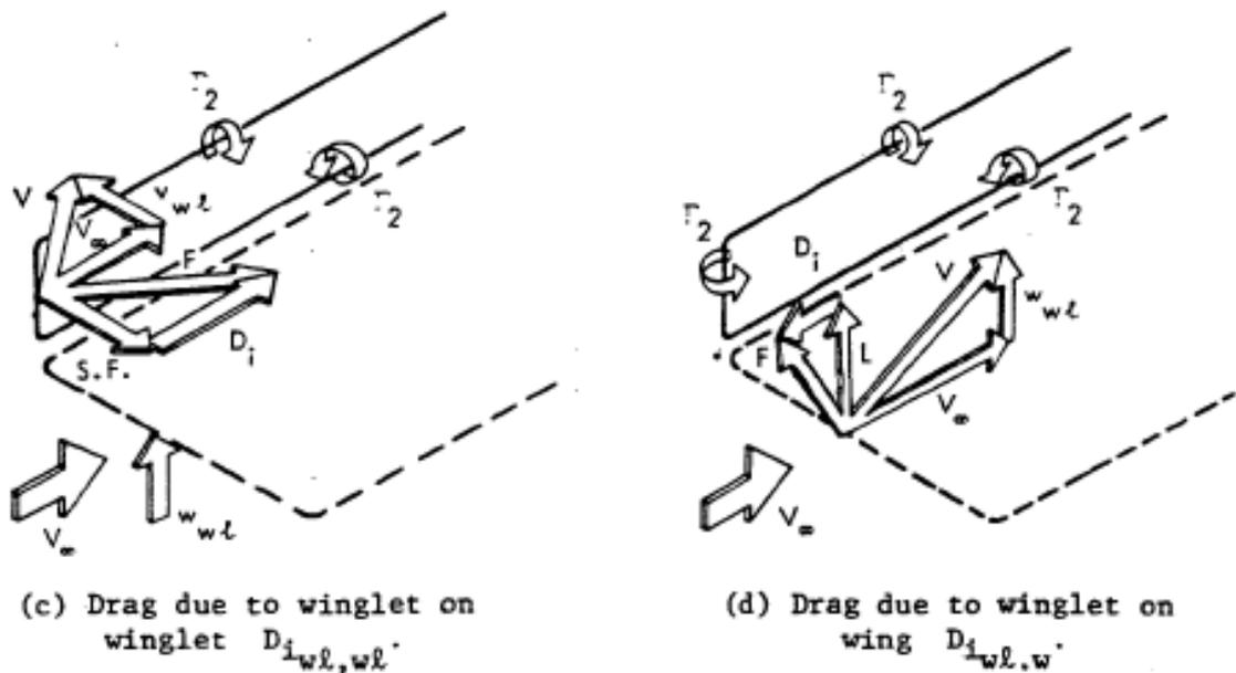
**Figure 2.7 - Sources of induced drag for a wing-winglet configuration (Gall, 1984)**
