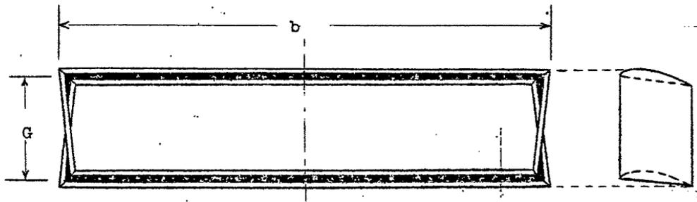
**Figure 2.5 - Prandtl's best wing system, front and side views (Prandtl, 1924)**
