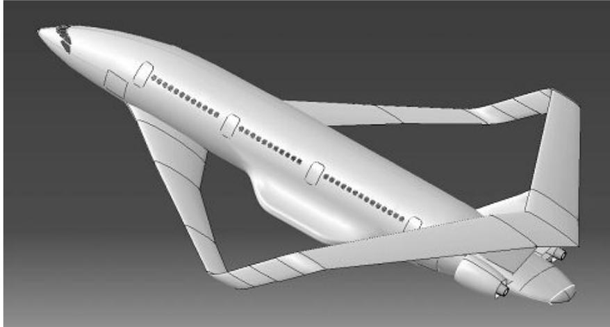
**Figure 2.11 - Parametric view of preliminary study for a 250 PAX box-wing aircraft (Frediani A, 2005)**
