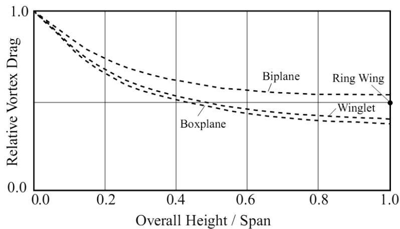
**Figure 2.4 - Induced drag variation with allowable height for nonplanar systems (Kroo I. , 2005)**
