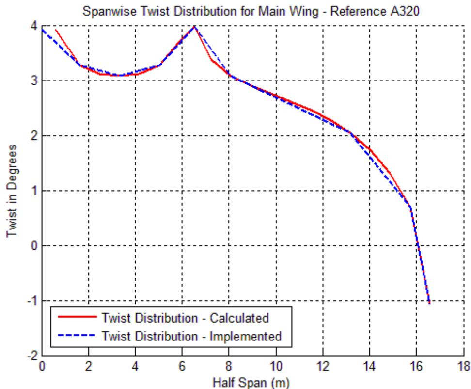
**Figure 4.9 - Spanwise twist distribution for reference A320**
