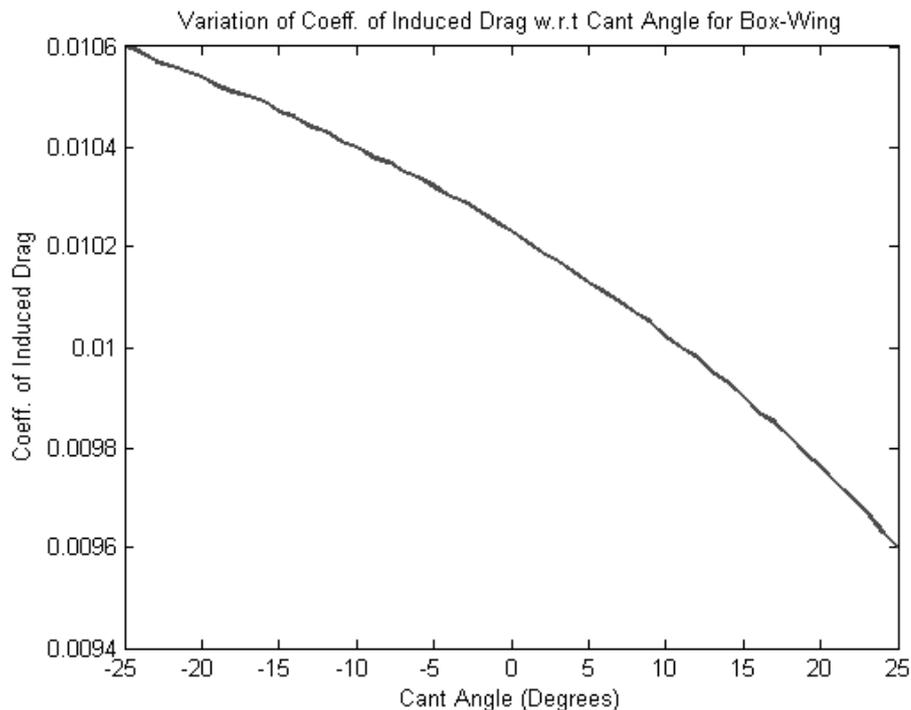
**Figure 4.4 - Variation of coefficient of induced drag with winglet cant angle**
