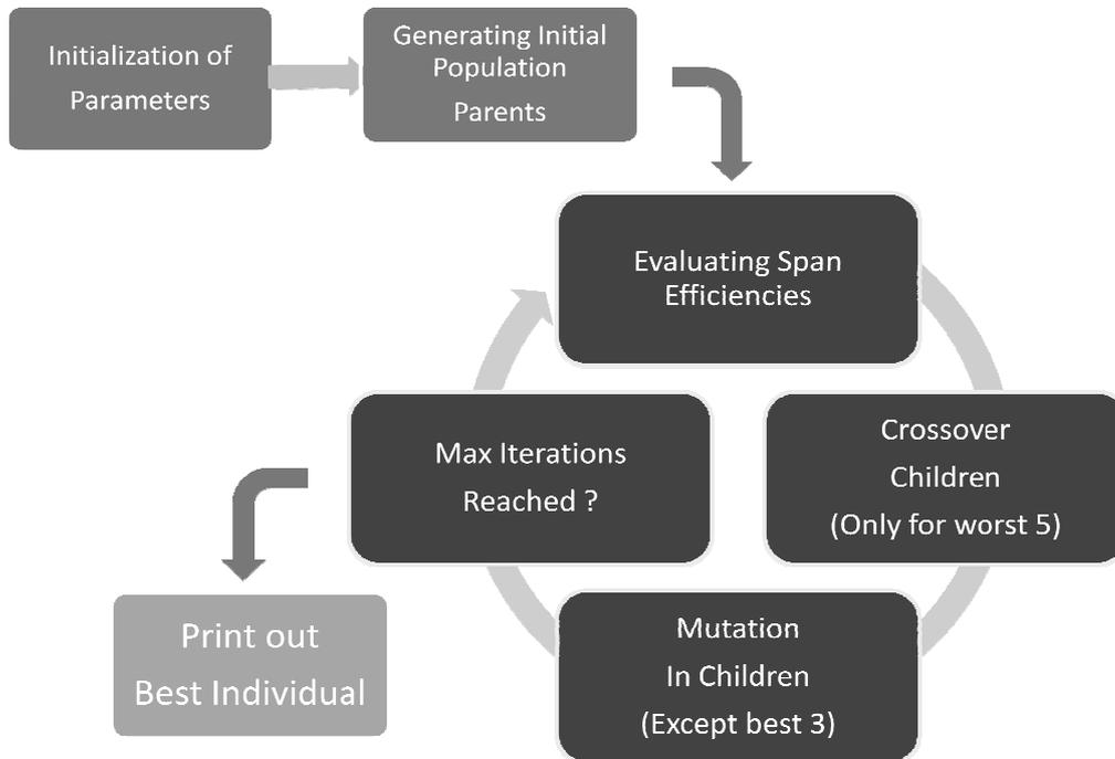
**Figure 4.5 - Canonical genetic algorithm flow chart**
