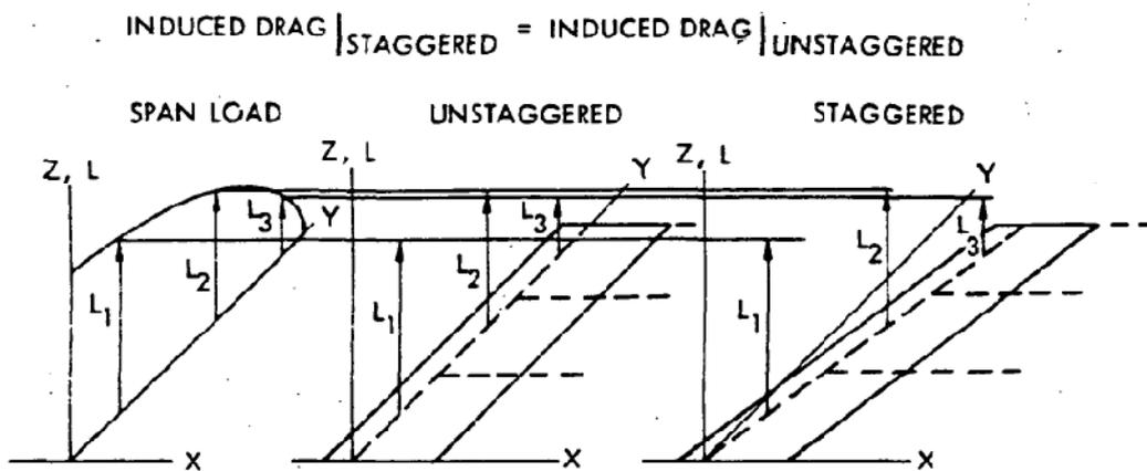
**Figure 2.6 - Illustration of Munk's stagger theorem (Gall, 1984)**
