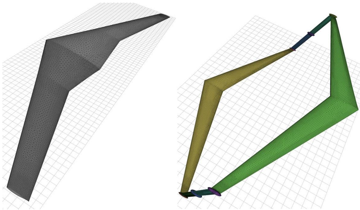
**Figure 5.1 - Surface mesh created in SUMO for reference A320 wing (Right) selected box-wing configuration (Left)**
