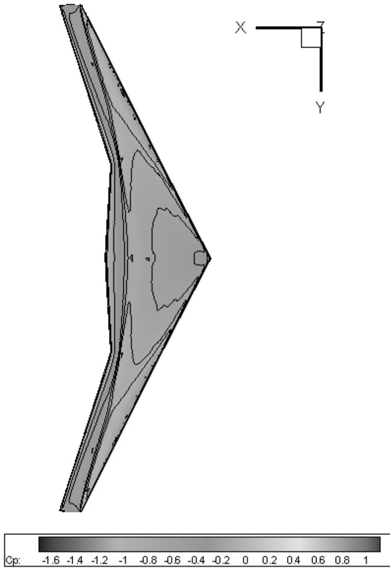
**Figure B.5 -  $C_p$  distribution for reference A320 wing (Top View)**
