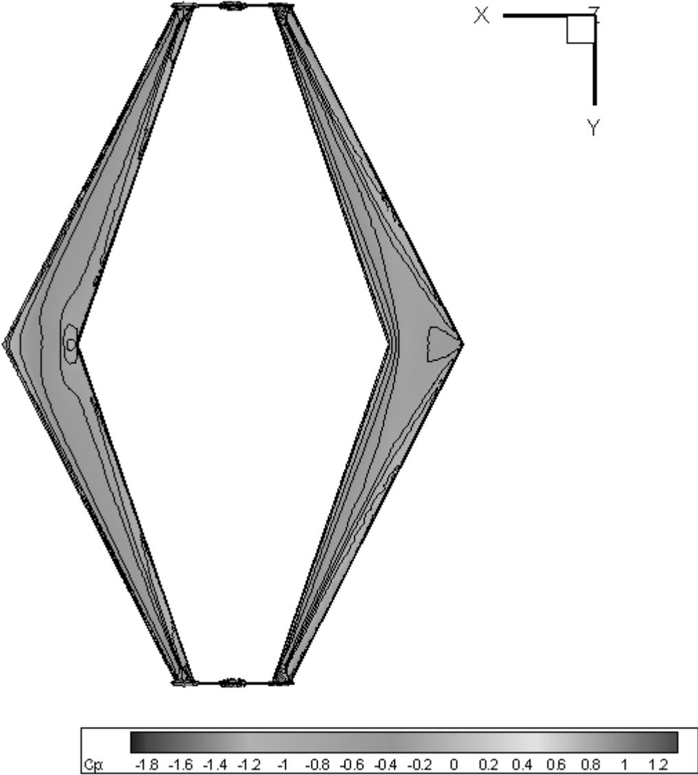
**Figure B.3 -  $C_p$  distribution of box-wing configuration (Top View)**
