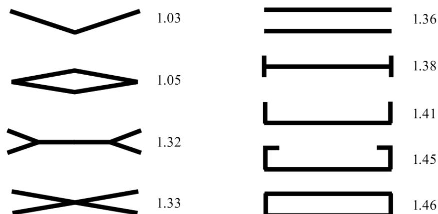
**Figure 2.3 - Span efficiencies for various optimally loaded nonplanar system ( $h/b=0.2$ ) (Kroo I. , 2001)**
