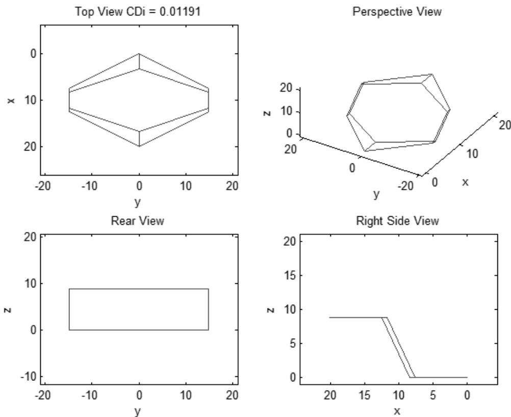
**Figure 4.7 - Selected box-wing configuration for CFD study**
