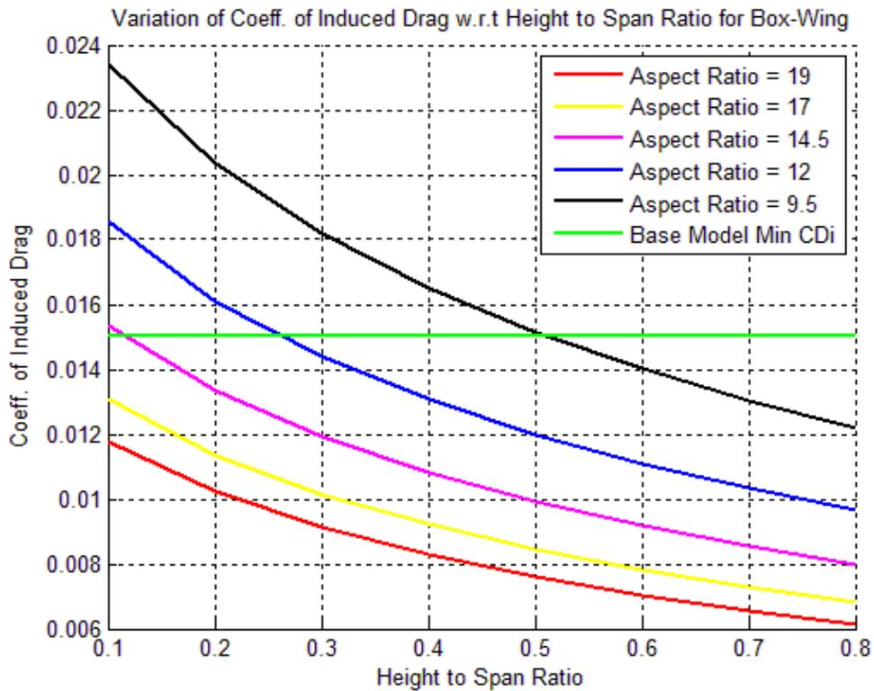
**Figure 4.2 - Variation of induced drag with height to span ratio**
