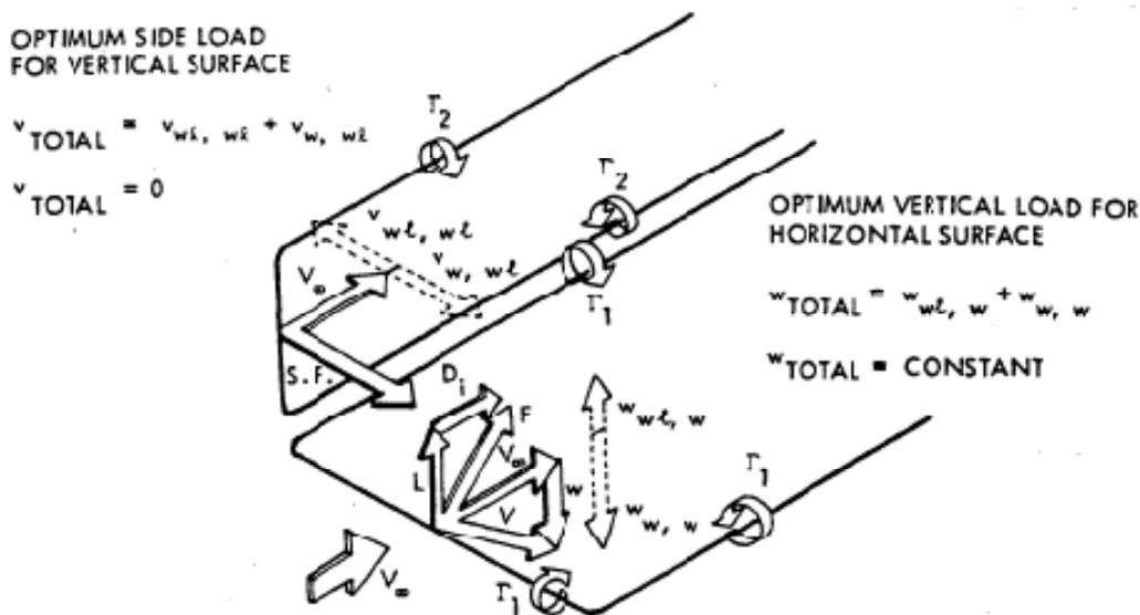
**Figure 2.8 - Combined sources of induced drag for wing-winglet configuration (Gall, 1984)**
