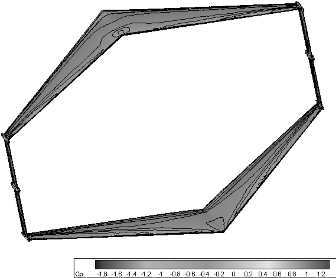
**Figure B.4 -  $C_p$  distribution of box-wing configuration (Asymmetric View)**
