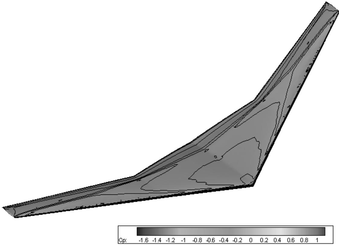
**Figure B.6 -  $C_p$  distribution for reference A320 wing (Asymmetric View)**
