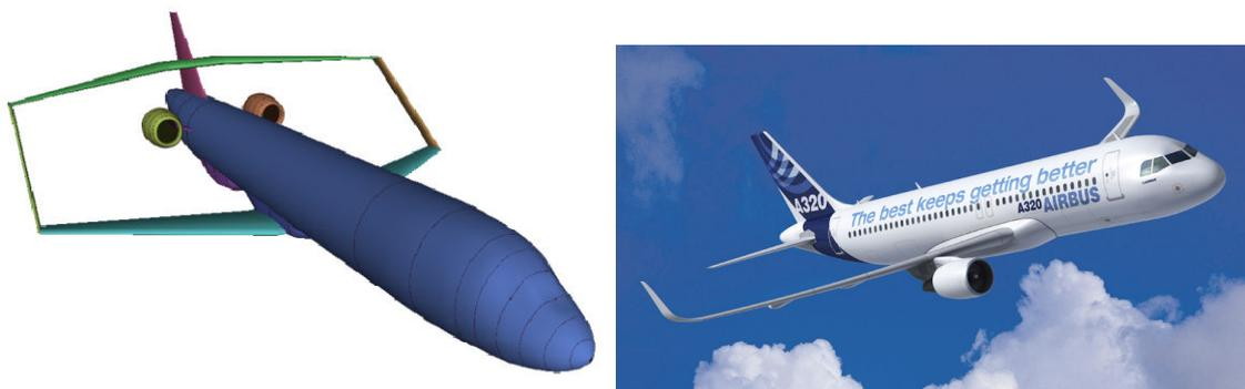
**Figure 6.1 - Box-Wing variant of A320 (Left) and Airbus A320 (Courtesy Airbus) (Right)**
