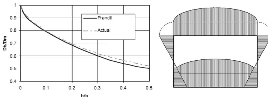
**Figure 2.10 - Comparison between Frediani's and Prandtl's solution (Left). Lift distribution for box-wing (Right)**
