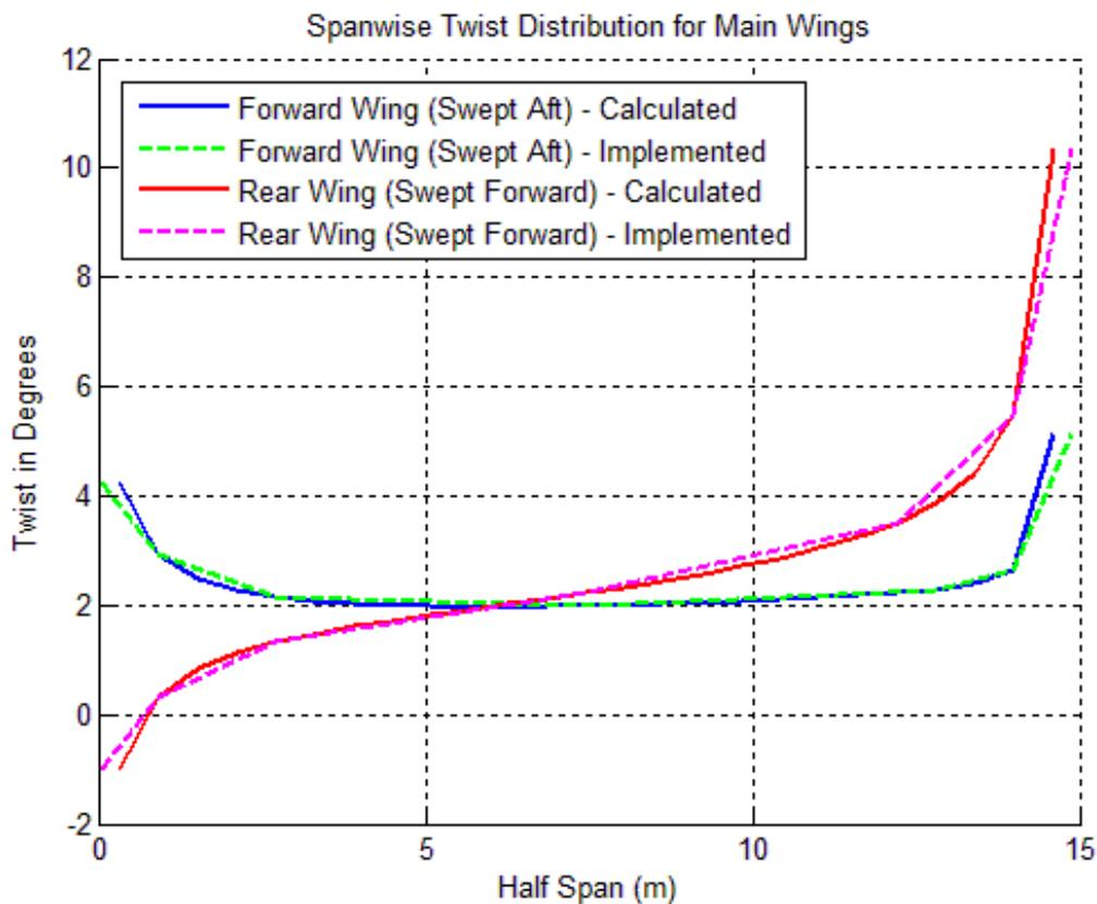
**Figure 4.10 - Spanwise twist distribution for main wings of selected box-wing configuration**
