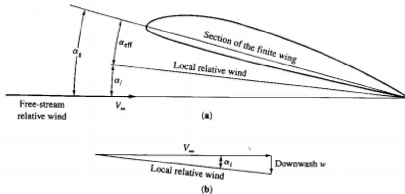
**Figure 2.2 - Illustration of induced and effective angle of attack caused by downwash (Anderson J. D., 1999)**
