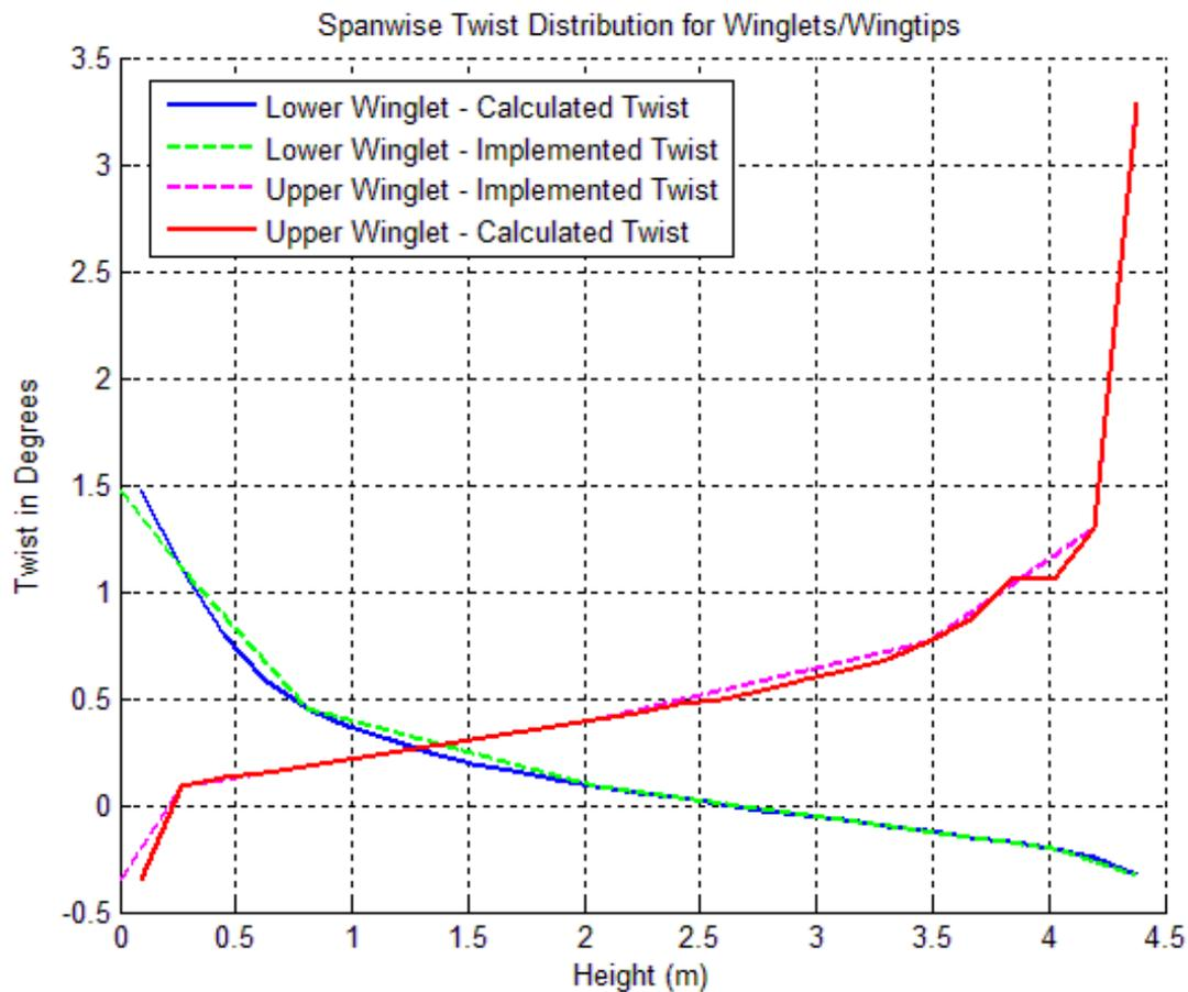
**Figure 4.11 - Spanwise twist distribution for winglets of selected box-wing configuration**
