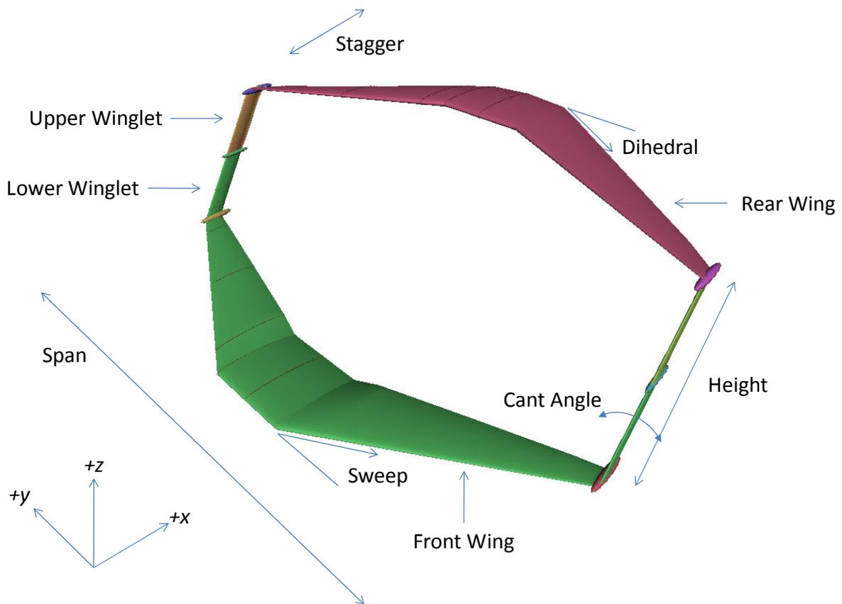
**Figure 3.1 - Box-Wing geometry**
