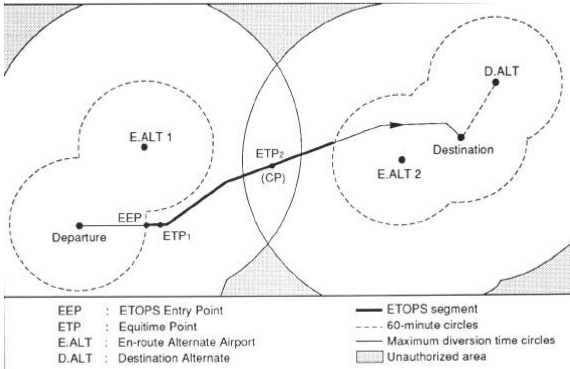
**Fig. 5 ETOPS Area Of Operation [2]**
