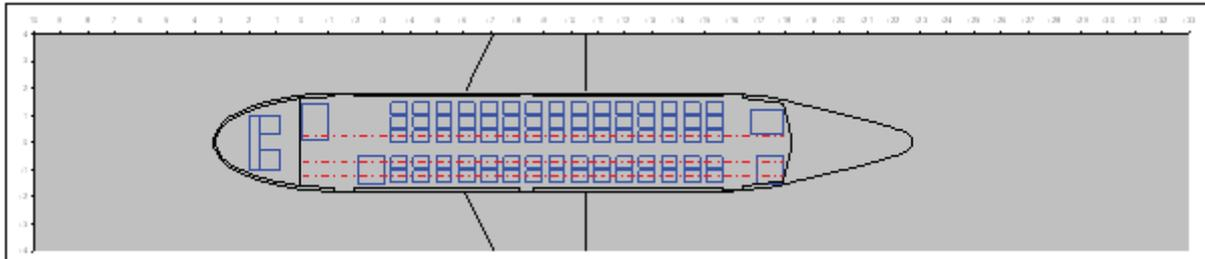
Figure 5: PreSTo cabin floor plan of Fairchild-Dornier 728 re-design
