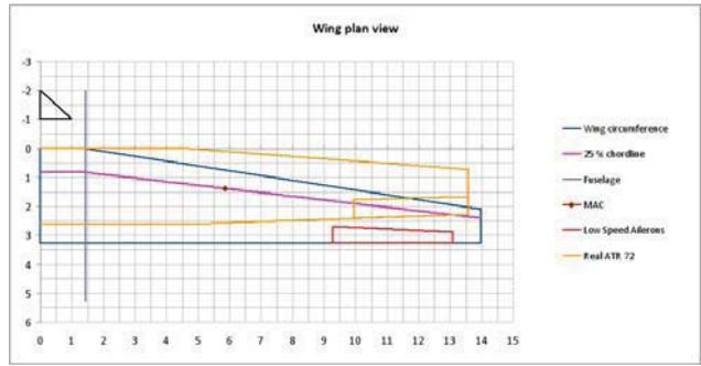
FIG 16. Wing shape V04 to real ATR 72
