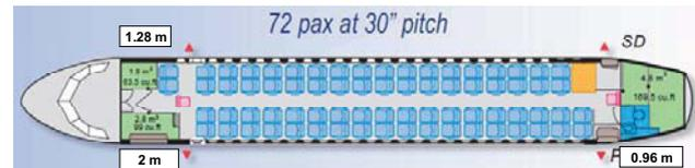
FIG 12. Real ATR 72 floor plan (72 pax)
