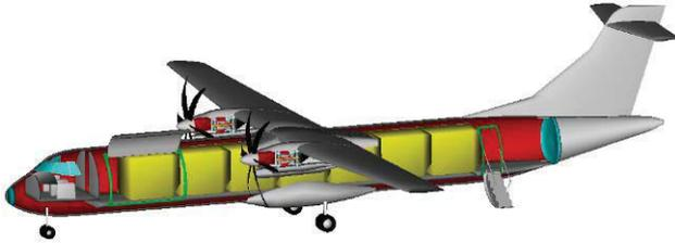
FIG 8. PrADO model of the original ATR 72 full freighter version
