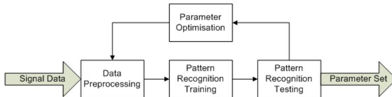
Figure 2: PAHMIR condition monitoring process with optimization
