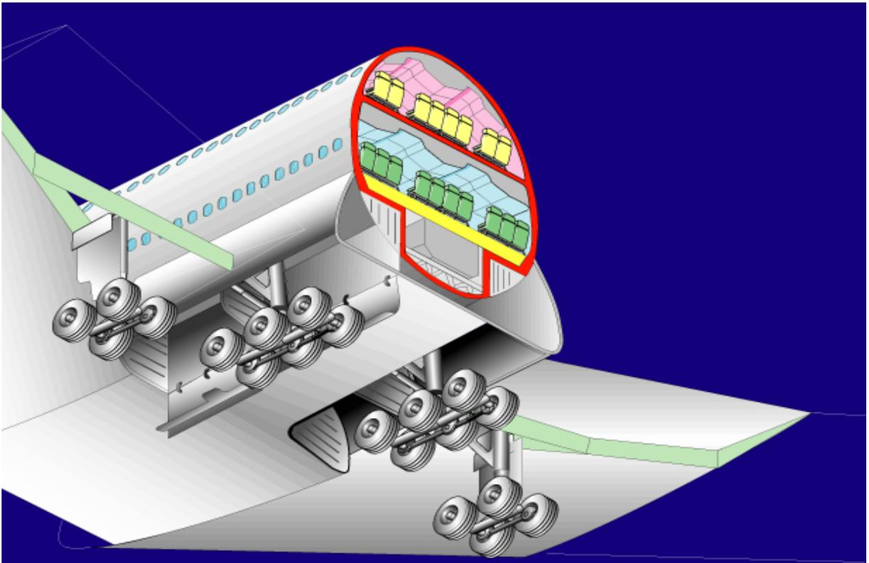
Fig. 12.10 A380 main landing gear with rearward retracting body gear
