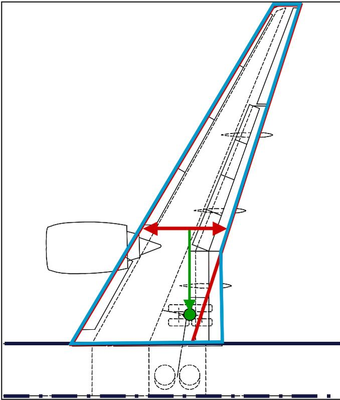
**Fig. 12.6.** Kinked wing trailing edge to give space for a wing mounted landing gear.
