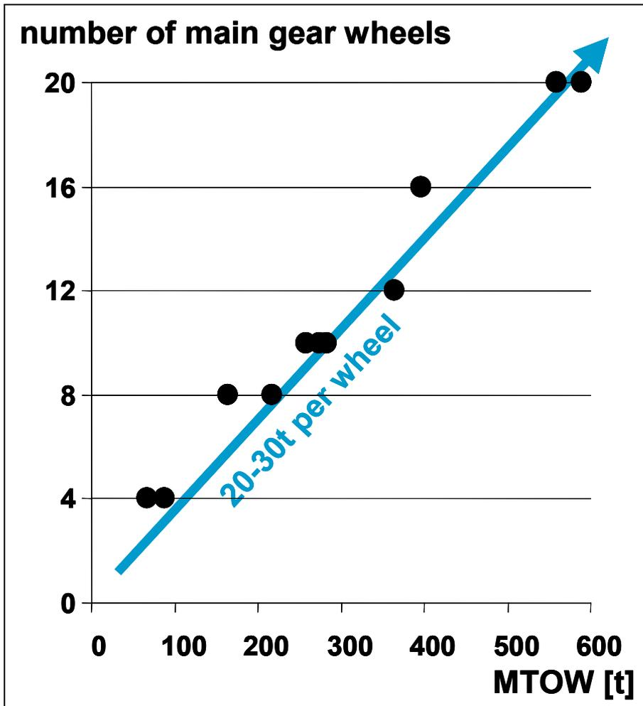
Fig. 12.12 Empirical diagram of number of wheel vs MTOW
