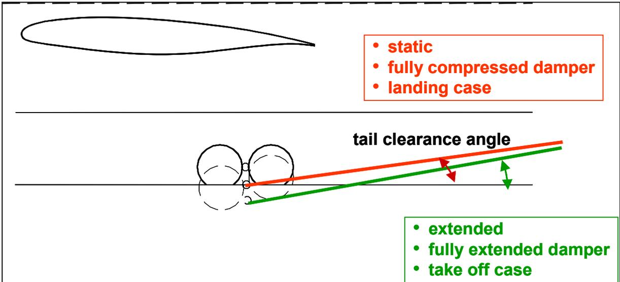
Fig. 12.4 Static and extended tail clearance angle
