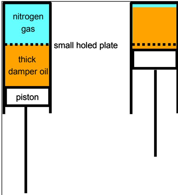
**Fig. 12.11** Principle sketch of oleo element in telescopic landing gear leg.
