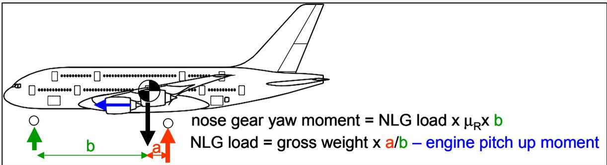
Fig. 12.5. Nose gear load drivers
