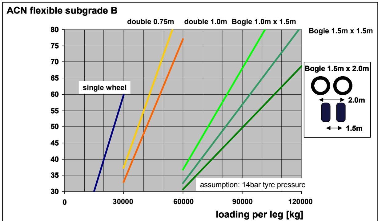
Fig. 12.7 Exemplary ACN effects of wheel and axle spacing
