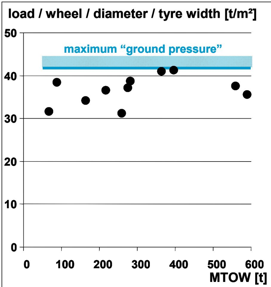
**Fig. 12.13** Empirical diagram to show average MTOW load per tire number per tire size
