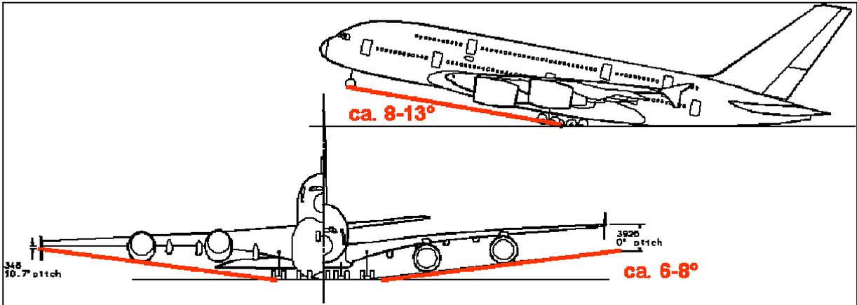
**Fig. 12.3** Tail clearance and bank clearance angle
