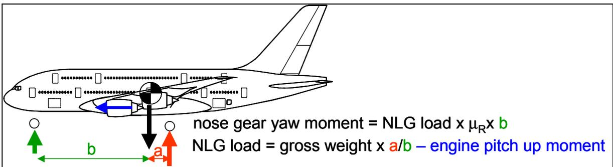
Fig. 12.5. Nose gear load drivers
