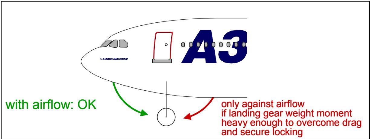
Fig. 12.9 Free fall with help of the airflow
