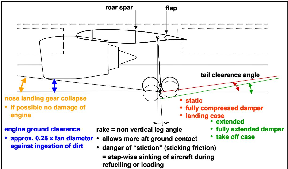
**Fig. 12.14** Drivers on main landing gear length and position on conventional aircraft
