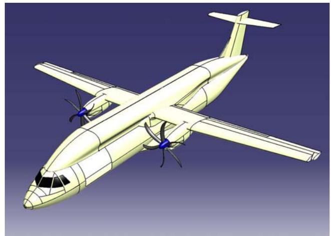
FIG 4. Regional cargo aircraft with fuel stores mounted on top of the fuselage
