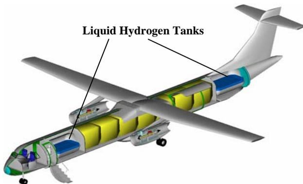
FIG 7. Hydrogen-powered regional cargo aircraft with fuel tanks inside the fuselage
