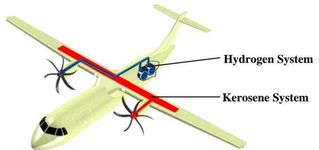
FIG 9. Hybrid-powered demonstrator aircraft
