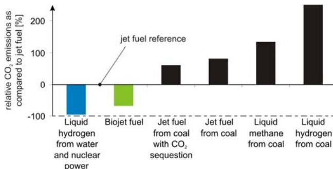
FIG 3. Relative carbon dioxide emissions of different alternative fuels over their whole life-cycle compared to conventional kerosene (based on IATA, 2008)
