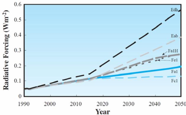
FIG 1. Estimates of the globally and annually averaged total radiative forcing (without cirrus clouds) associated with aviation emissions under different scenarios to 2050 (Penner et al., 1999), with Fa1 as the reference scenario that assumes improvement in fuel efficiency and mid-range economic growth
