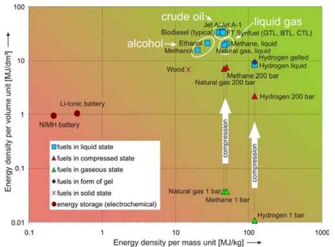
FIG 2. Volumetric and gravimetric energy contents of different fuels and batteries on a double logarithmic scale (based on Sieber, 2009)
