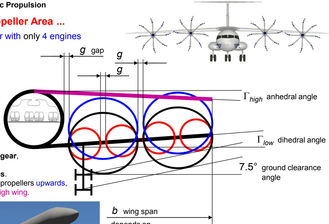
length of landing gear, depends on number of engines. Alternatively: shift propellers upwards, maybe mount on high wing.
