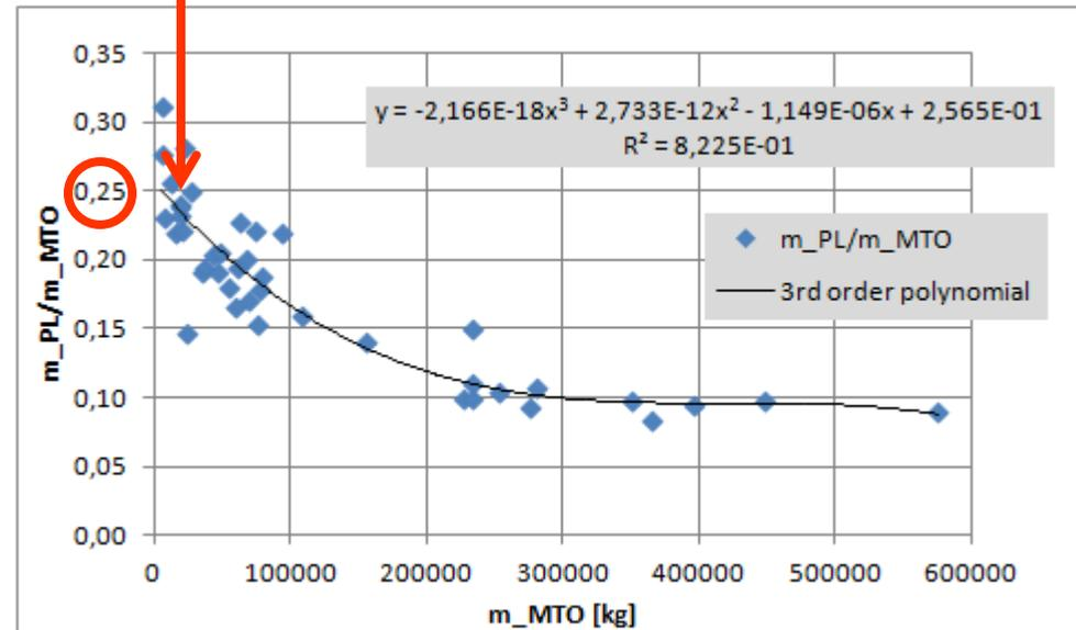
Payload,  $m_{PL}$  calculated from "typical number of seats" from manufacturers seat layout and 93 kg/seat. Data points represent passenger aircraft most frequently in use with 19 seats or more. Note: Although the regression is quite good, physically  $m_{PL}/m_{MTO}$  is a function of range.
